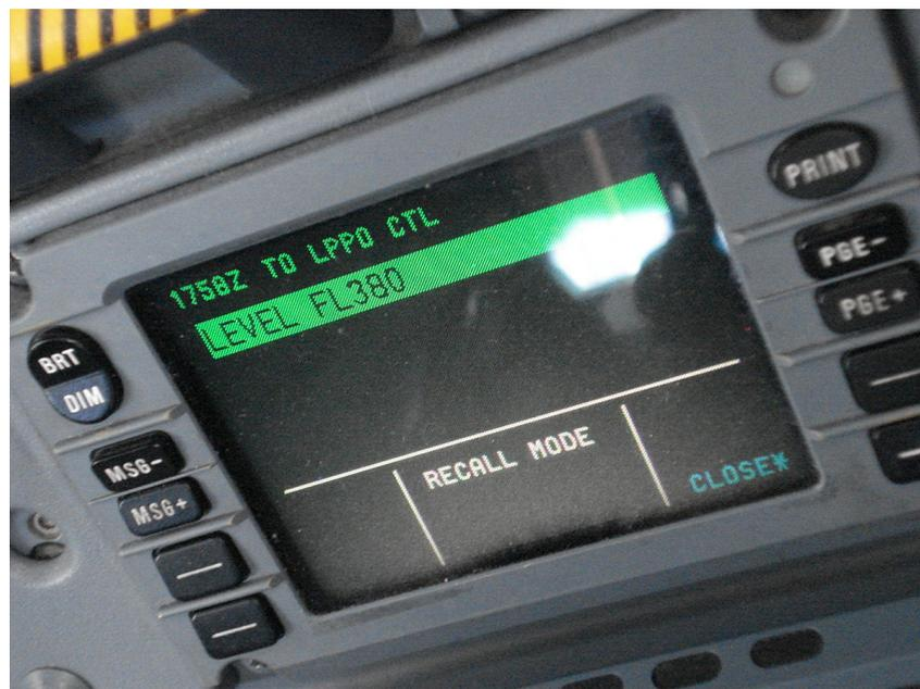
FIGURE 2.2: DCDU Airbus A330
