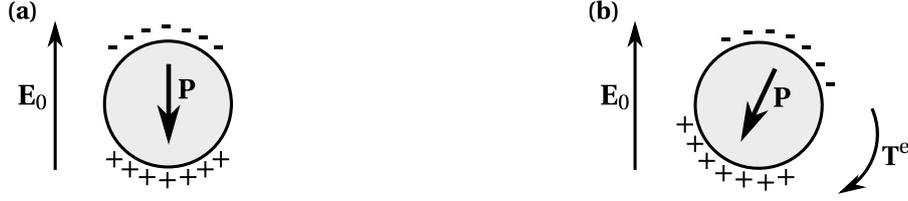
**Figure 1.2** – Emergence of the Quincke rotation. (a) Electric charges accumulate at the particle-liquid interface and result in a dipolar surface distribution. (b) When a small rotational perturbation tilts the dipole  $\mathbf{P}$ , a net electric torque  $\mathbf{T}^e$  amplifies the initial perturbation.
