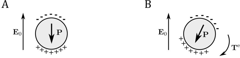
**Figure 1.21** – Emergence of Quincke rotation. **A**– Electric charges accumulate at the particle-liquid interface and result in a dipolar surface distribution. **B**– A small rotational perturbation tilts the dipole  $\mathbf{P}$ , thereby inducing a net electric torque  $\mathbf{T}^e$  which amplifies the initial perturbation.
