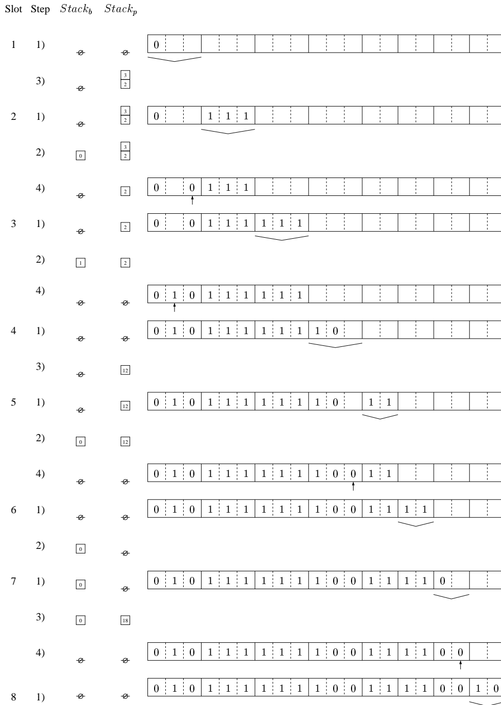
FIG. 6.4 – Example 6.6.3 : Encoding of sequence a_1a_4a_5a_2a_3a_3a_1a_2 using code C_7 and algorithm SMA-stack.
