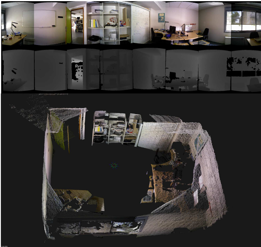
Figure 3.19: Top to bottom: photometric and geometric maps obtained from the device of figure (3.15) with their corresponding point cloud obtained by the spherical projection described in section (3.7.2)
