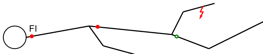
Figure II.1: Fault on a lateral between two FIs
