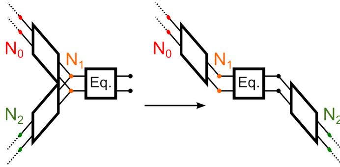
Figure III.13: Insertion of the lateral in the feeder
