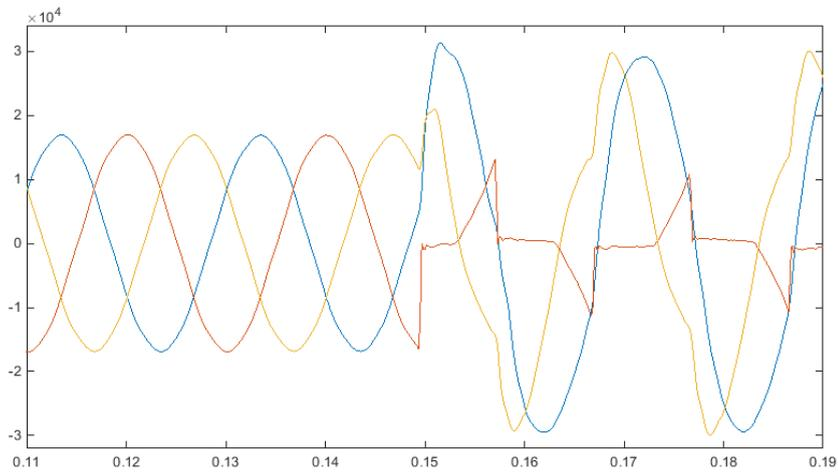
Figure III.19: Phase voltages during arc fault
