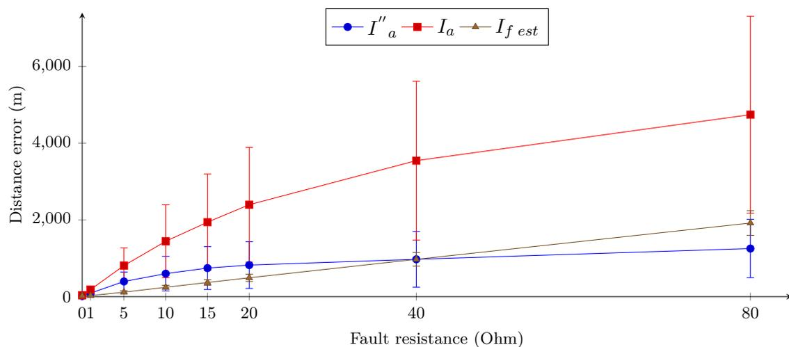
Figure IV.10: Superposition of the results for  $I''_a$ ,  $I_a$  and  $I_{f\ est}$  - Mean distance error (m), in absolute value, on all fault locations for each fault resistances and the standard deviations associated
