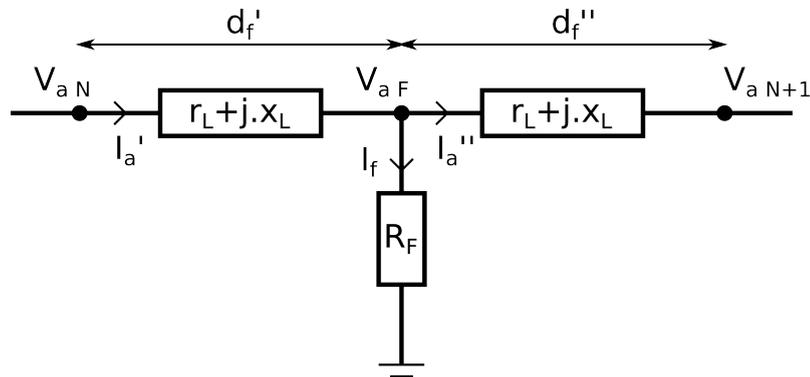
Figure III.16: Electrical diagram of the faulted phase
