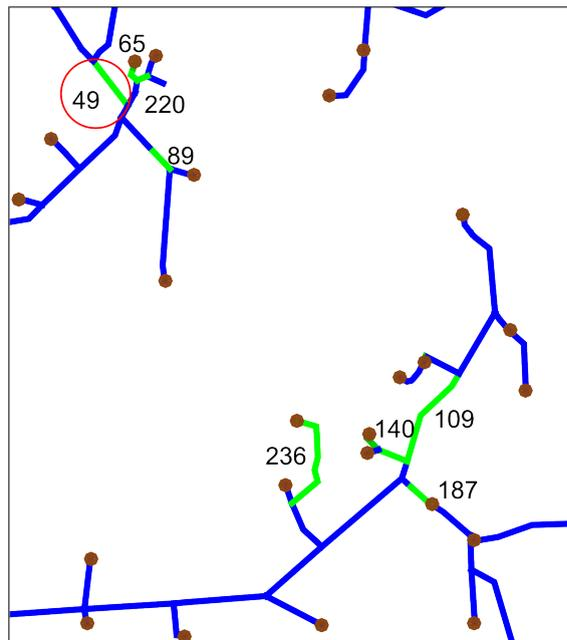
Figure F.1: Illustration of the eight fault locations found by the algorithm in the case of the fault  $F3 - 5 \Omega$  (green sections)
