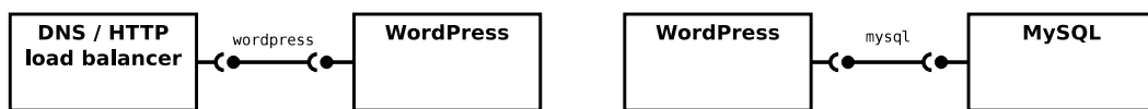
(a) The binding between a load balancer instance (HTTP or DNS based) and a WordPress instance on port wordpress . (b) The binding between a WordPress instance and a MySQL instance on port mysql .
