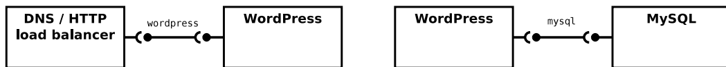
(a) The binding between a load balancer instance (HTTP or DNS based) and a WordPress instance on port wordpress . (b) The binding between a WordPress instance and a MySQL instance on port mysql .
