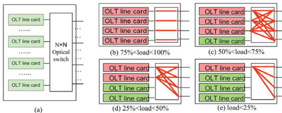
Figure 5.9: OLT with Optical Switches (Zhang, et al., 2011)
