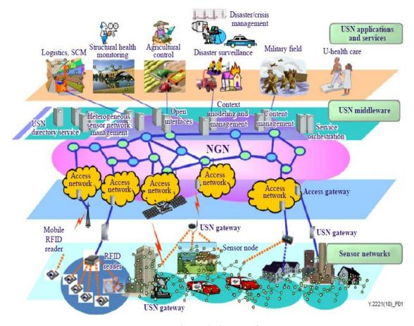
Figure 3.1: Schematic layers of USN [1]
