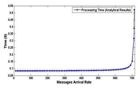
Figure 6.5: The processing time of VANET applications on the IMS servers
