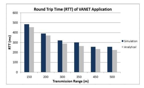
Figure 6.6: Round Trip Time comparison between the analytical and simulation results of the proposed VANET application at (L = 2 km)
