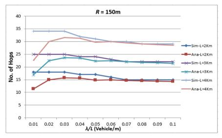
Figure 5.3: Comparison of number of hops of different road lengths at a transmission range (R = 150m)
