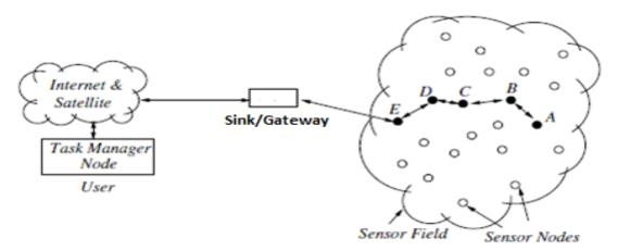
Figure 2.1: Sensor nodes scattered in a sensor field [14]
