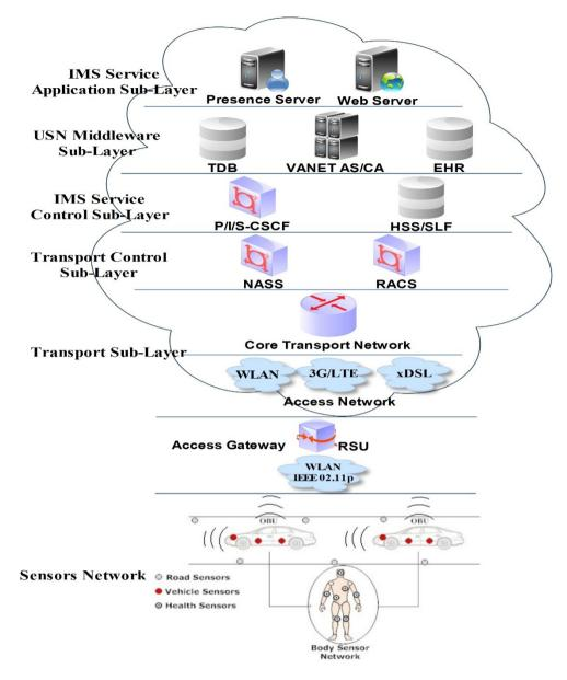
Figure 6.1: Next generation VANET network architecture
