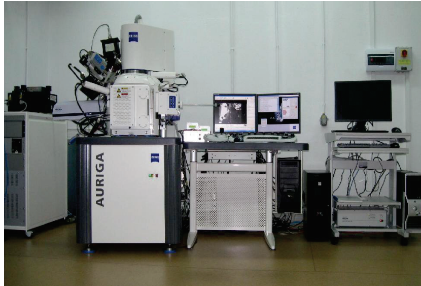
Figure 2-25: AURIGA CrossBeam Workstation (FIB-SEM) from Carl Zeiss [41] for the preparation of FIB sections from irradiated powellite single crystals
