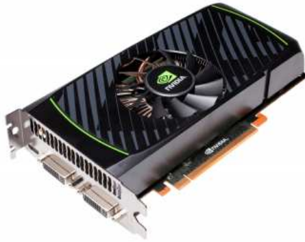
FIGURE 3.13: Graphics Processing Unit.
