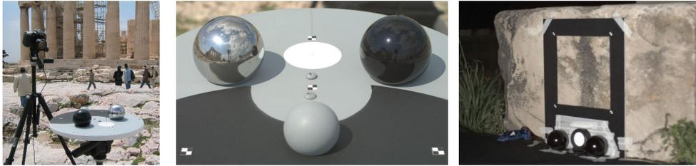
**Figure 2.19:** Acquisition devices use to capture BRDF.
