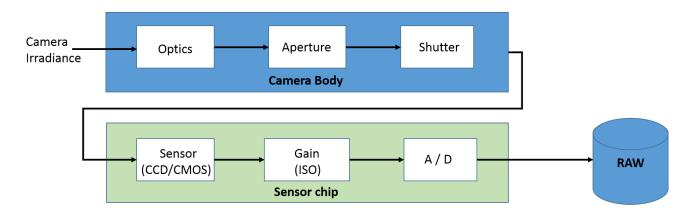
Figure 2.2: DSLR pipeline as described in [Szeliski, 2010b].
