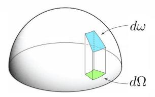
Figure 2.5: Element of solid and projected solid angle.
