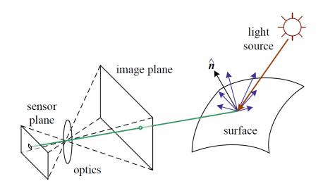
**Figure 2.1:** A simplified model of photometric image formation. Light is emitted by one or more light sources and is then reflected from an object's surface. A portion of this light is directed towards the camera. This model ignores multiple reflections, which occur in real-world scenes. [Szeliski, 2010a]
