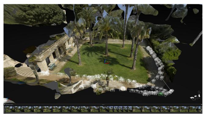
**Figure 2.4:** Screenshot of the photofly reconstruction of an outdoor scene showing camera locations, Refer to the dataset section to get more details.
