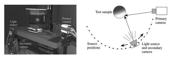
**Figure 2.29:** [Marschner *et al.*, 2000] setup using 2 cameras, a light source and the test sample.
