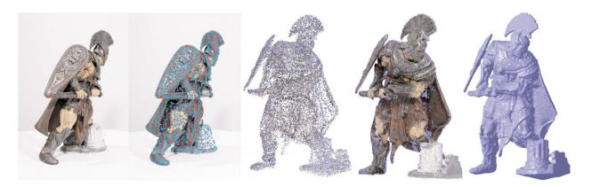
**Figure 2.3:** Overall approach from [Furukawa and Ponce, 2007]. From left to right: a sample input image; detected features; reconstructed patches after the initial matching; final patches after expansion and filtering; polygonal surface extracted from reconstructed patches.
