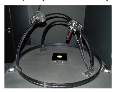
**Figure 2.28:** A gonioreflectometer measuring the BRDF of a planar sample by sampling the double hemisphere of incoming/outgoing radiance using a directional light source. [Li *et al.*, 2005]
