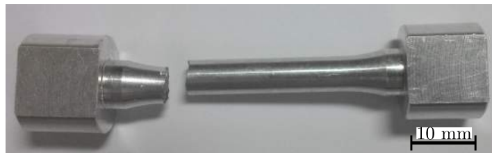
Fig. B.1: Image showing an example of a post-mortem as-machined specimen which failed at one of the junctions.
