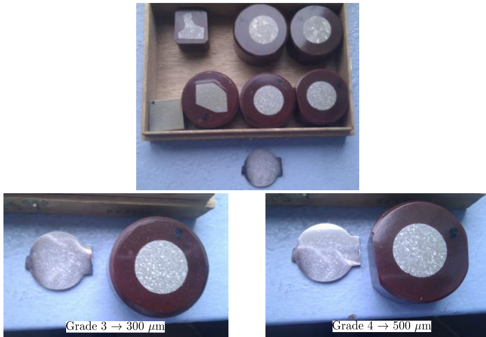
Fig. 1.18: Grain microstructure was revealed by using a chemical etchant on a mirror polished sample. Comparison between this sample and CTIF rating charts enables determination of the average grain size.
