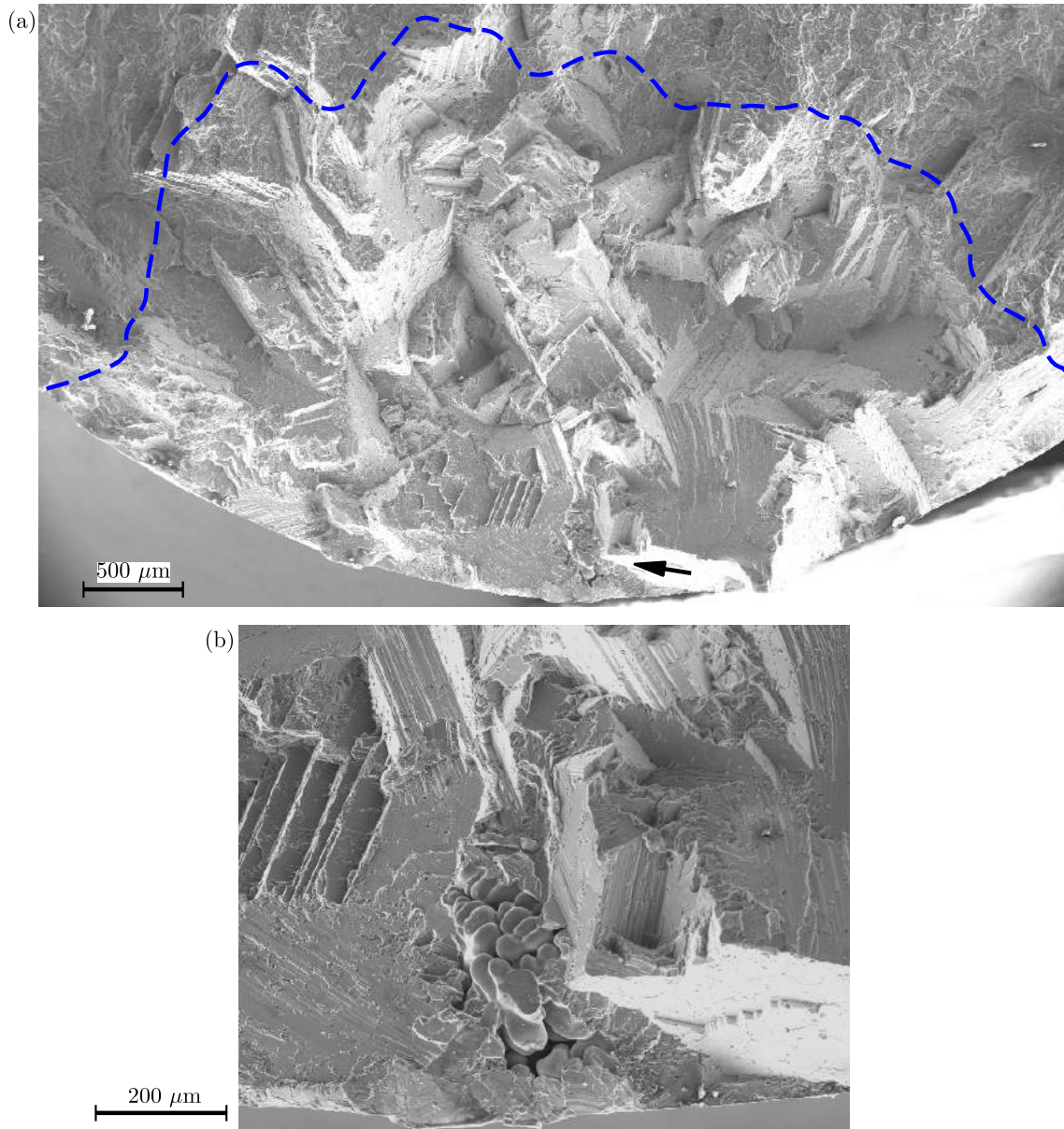
Fig. 3.16: (a) SEM observations on the fracture surface of ENSMA-SNV-03 specimen (vacuum, N_f = 3\,356\,341 cycles, \sigma_{\max} = 133 MPa, Artificial Defect \sqrt{A} = 278 μm). Only Region II propagation is observed. (b) Higher magnification on the first propagation stages from a surface microshrinkage, close to the region indicated by the black arrow.
