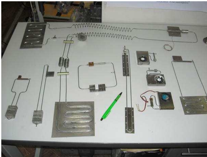
(d) LHP produced by Maydanik’s research team at the Institute of Thermal Physics
