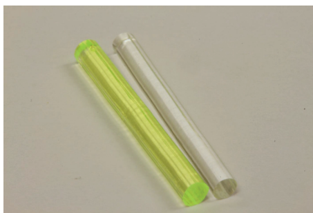
Figure 6.1: Two LuAG fibers of \varnothing 2 mm and length 2 cm. The right sample is undoped whereas the sample on the left was doped with 0.1 at.% of Cerium.
