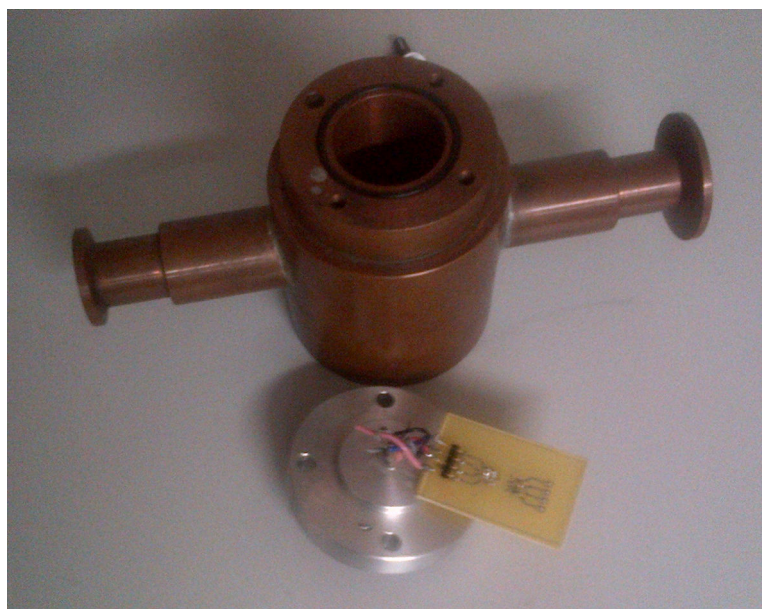
FIGURE A.3 – Enceinte isobare
