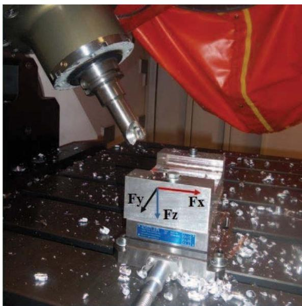
Fig. 6-3 Experimental setup
