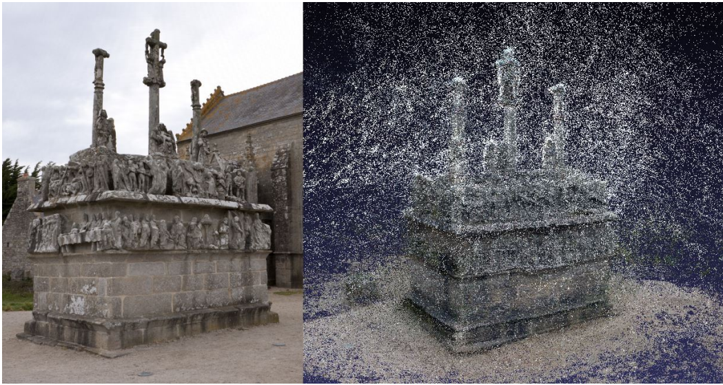
Figure 1.2: Multi-view stereo. Left: One of the 27 images taken from a calvary. Right: Point cloud reconstructed by Vu et al. [VKLP09], containing a significant amount of outliers. Images courtesy by Vu et al. [VKLP09].
