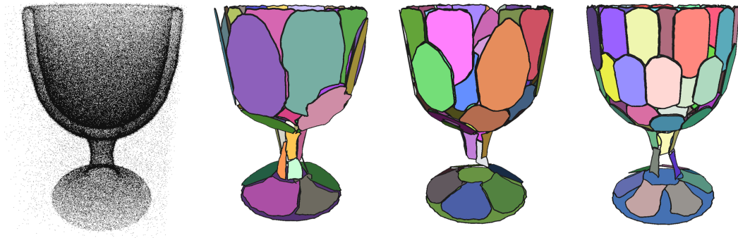
Figure 3.5: Multiscale Planar Abstraction. Left: Input point cloud of a goblet with outliers and noise. Middle left to far right: Planar abstraction with varying fitting tolerance from coarse to fine: 1%, 0.5% and 0.25% of bounding box diagonal.
