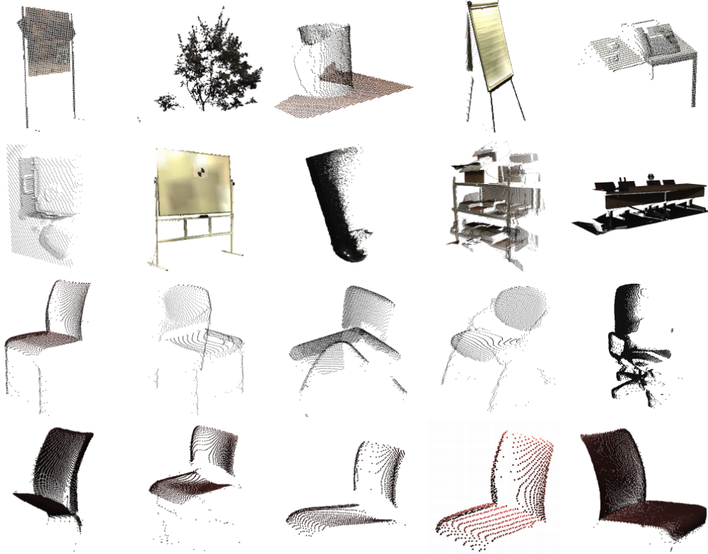
Figure 3.10: Indoor objects. We acquired 20 indoor objects with a Leica Scanstation P20 laser scanner. The sampling of the objects is heterogeneous and partly anisotropic. The lower 10 objects are labeled as chairs whereas the upper ten objects are labeled as non chairs.
