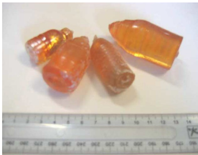
Fig. 2.2. Photo of the \text{ZnMoO}_4 crystals 20 mm–30 mm in diameter and 30 mm–40 mm in height grown by the Czochralski technique in 2009 year [158]. The scale is in centimeters.
