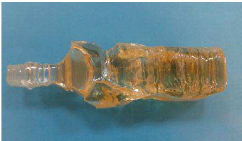
Fig. 2.7. Photo of the \text{Zn}^{100}\text{MoO}_4 crystal boule enriched in ^{100}\text{Mo} to 99.5%. The boule with the mass of 170.7 g and length of 95 mm was grown for the first time by using low-thermal-gradient Czochralski technique in the Nikolaev Institute of Inorganic Chemistry.
