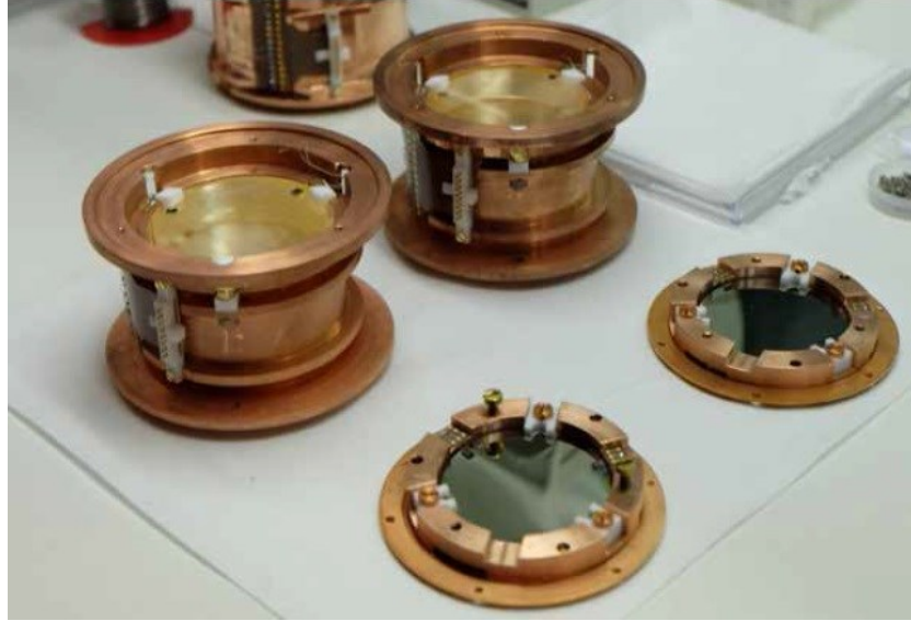
Fig. 2.17. Photo of the scintillating bolometers based on 336 g and 334 g \text{ZnMoO}_4 crystals of advanced quality with their ultrapure Ge photodetectors.
