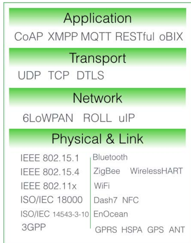
Figure 2.3: Related protocol and technologies to enable the IOT/WOT
