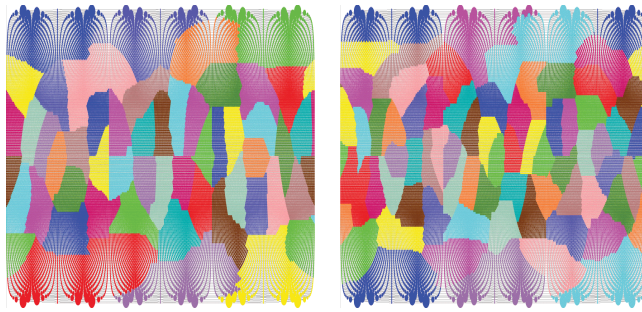
Figure 1.14: Mesh partitioning computed by the general purpose mesh partitioner Scotch for 54 domains (optimal case for Pangolin, left) and 72 domains (sub-optimal case for Pangolin, right). Each color corresponds to a subdomain (the same color can be used for different partitions). The grid contains 48 600 cells and is shown in latitude–longitude coordinates.
