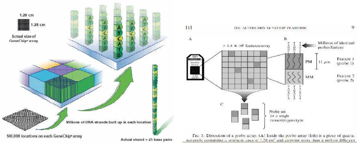
Figure 2.1: Affymetrix GeneChip array example: detailed schematic representation of a probe cell (left) (available at <http://www.vsni.co.uk/software/genstat/htmlhelp/marray/AffymetrixChips.htm>) and of a probe pair (right) [25].
