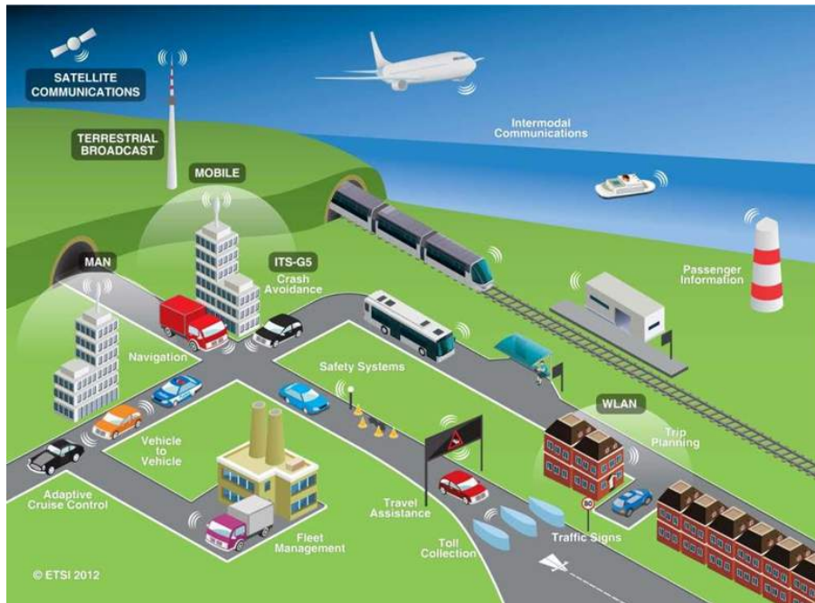
Figure 2.22: Intelligent Transportation Systems. A different set of radio transmission technologies and standard communication protocols makes the Inter-Vehicle Communication a possibility. The main goal to achieve is to improve safety on-roads and help saving lives. ©European Telecommunication Standards Institute 2008. Further use, modification, redistribution is strictly prohibited. ETSI standards are available from http://pda.etsi.org/pda/ .
