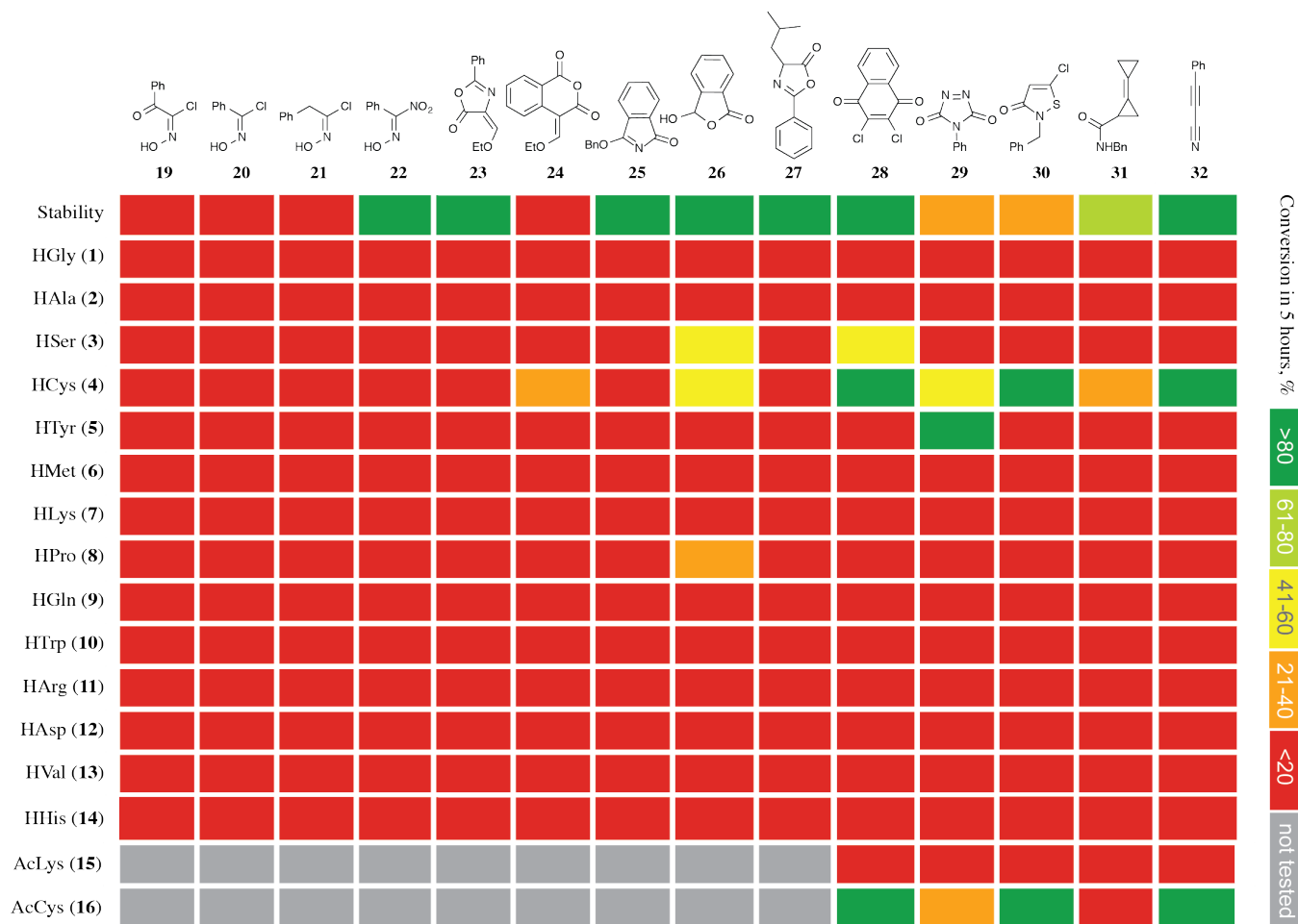
Fig. 100. Results of the screening. Reaction conditions: PBS (1x, pH 7.5), 25 °C, 1 mM concentrations of the reagent partners, 5 mM concentration of benzamide. Stability corresponds to the percentage of the non-hydrolysed probe.
