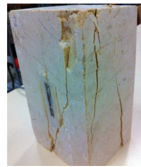
Figure III.3: rupture de pierre en compression
