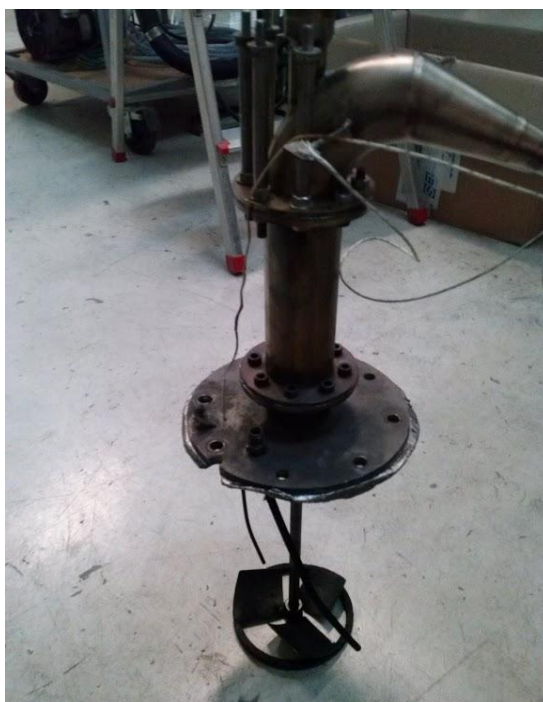
Photo 3-1. The mechanical mixer added to reactor
