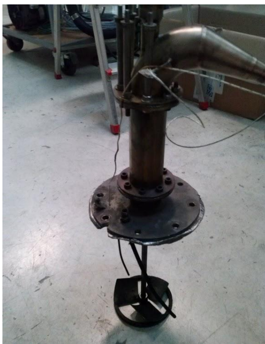
Photo 3-1. The mechanical mixer added to reactor
