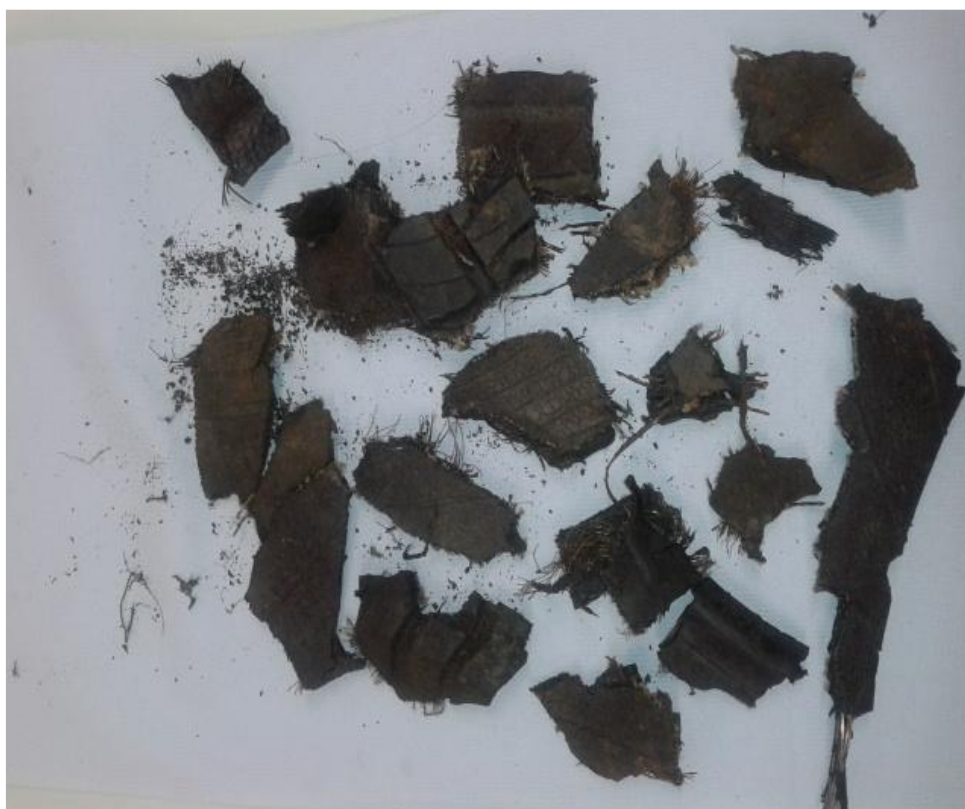
Photo 1 , Raw material scrap tires' pieces.
