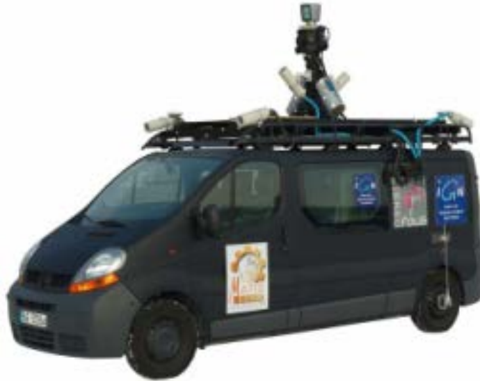
Figure 2.1 – IGN urban Mobile Mapping System equipped with a multi-camera system, turning Velodyne lidar, several high-precision lidars and a precise hybrid localisation system based on a GPS receiver coupled with an INS . Stereopolis vehicle is also equipped with a panoramic head and two pairs of stereo cameras. Source: Paparoditis et al. (2012).
