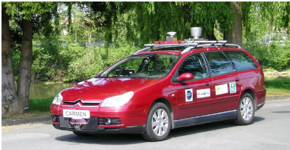
Figure 7.4 – Test vehicle Carmen with the lidar sensor in front.
