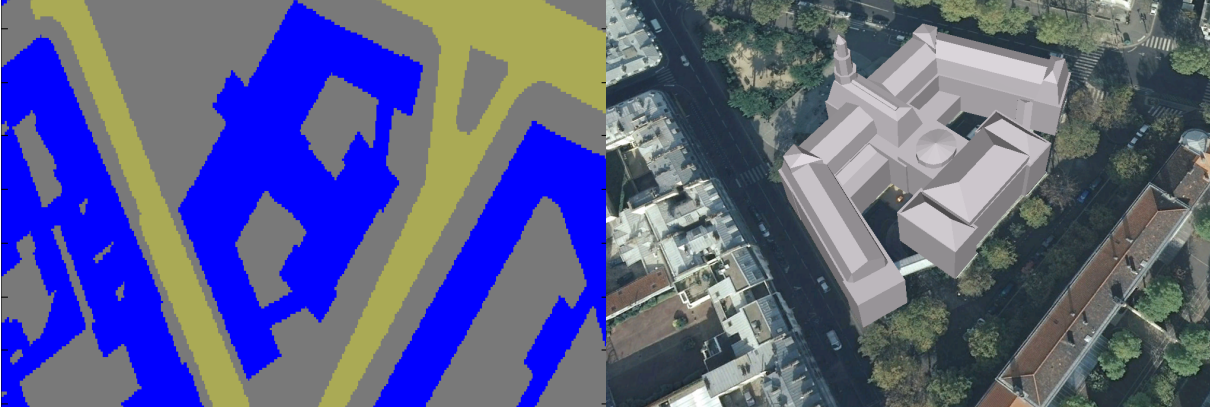
Figure 4.3 – Paris 12th district city-hall. Left: a portion of the constructed GISGrid obtained using data from IGN maps (Soheilian, Tournaire, et al. 2013). Right: 3D view of the area (Google 2014a). Colour code: blue – buildings, dark yellow – roads, grey – intermediate space.
