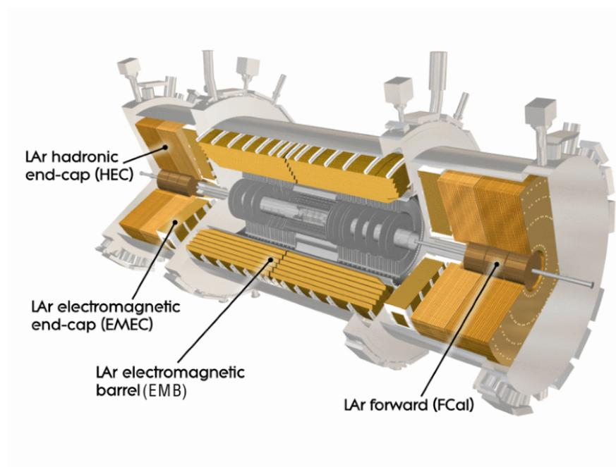
**Figure 2.12:** Pictorial representation of the ATLAS electromagnetic and hadronic calorimeters.
