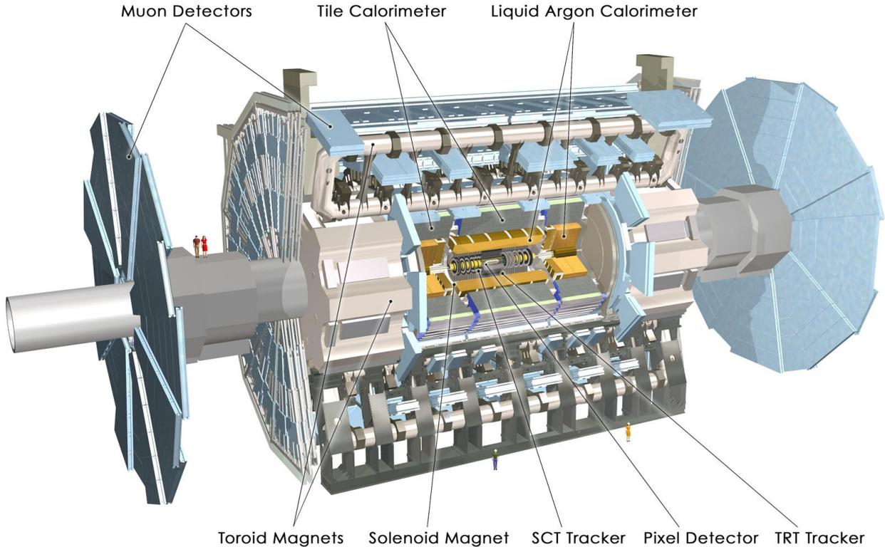
**Figure 2.6:** Schematic layout of the ATLAS experiment.
