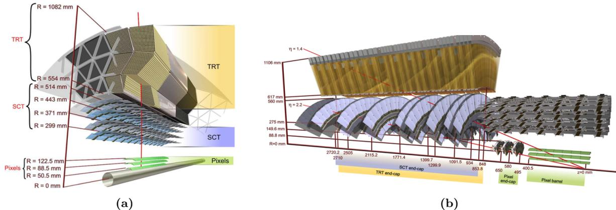
**Figure 2.9:** Pictorial sketch and localisation of the different modules comprised in the Inner Detector in the barrel (a) and in the end-caps (b) when traversed by a 10 GeV charged particles (red lines) for different pseudorapidity values ( $|\eta|=0.3, 1.4, 2.2$ ).
