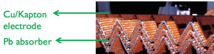
**Figure 2.14:** Accordion geometry of the electromagnetic calorimeter. Zoom on the internal structure: lead absorbers and LAr gaps representing the active medium are separated by insulating kapton foils.
