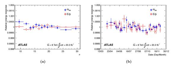
**Figure 4.3:** (a) - Energy response as a function of  $\mu$  normalised to its average quantity. (b) - Energy response as a function of time, normalised to its average quantity.
