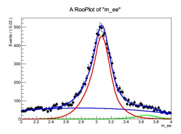
Figure 4.23: Invariant mass distribution of  $J/\Psi \to ee$  resonance, for electrons lying in the central  $\eta$  region, namely  $0 < \eta < 0.6$ . The final state histograms for  $J/\Psi$  events from data (black points) is compared with the sum of the signal (red line) and the  $J/\Psi_{2S}$  (green line) component (each parametrised with the sum two Crystal Ball functions), and the combinatorial background (blue line parametrised with a third order degree polynomial function).
