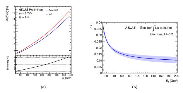
**Figure 4.11:** Inner detector (a) and calorimeter resolution (b) for electrons as a function of  $p_T$  and  $E_T$  in various pseudorapidity regions.
