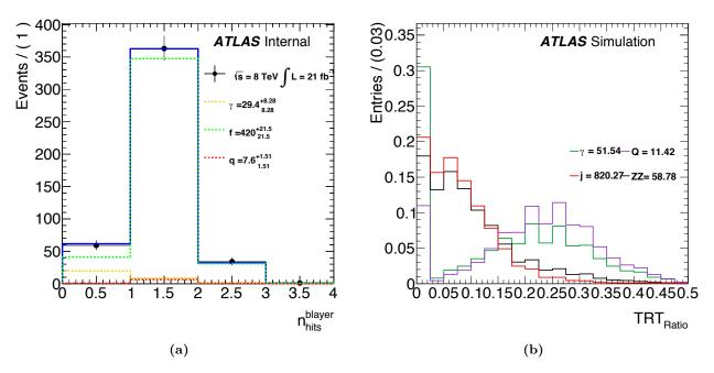
Figure 5.11: Fit to the number of b-layer hits and the TRT ratio of the number of high threshold to low threshold TRT hits for the background components in the 3l+X control region. The source of background electrons are denoted as: light flavour jets faking an electron (f), photon conversion ( $\gamma$ ) and electrons from heavy flavour quark semileptonic decays (q).
