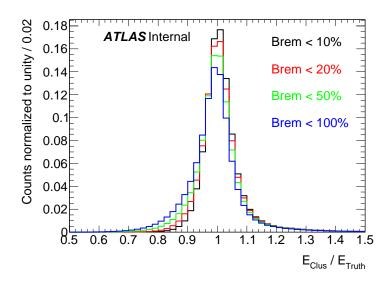
**Figure 4.22:** Evolution of the left tail of the energy response distribution for leading electrons in Monte Carlo  $J/\Psi \rightarrow ee$  decays.
