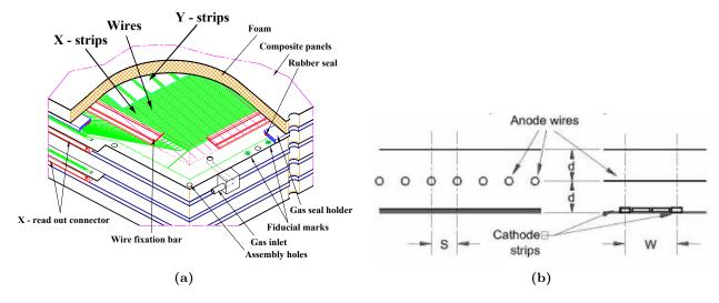
**Figure 2.20:** (a) Schematic drawing of a CSC chamber where structural components are indicated. (b) Sketch of a CSC chamber.
