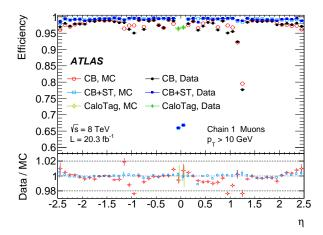
Figure 3.8: Muon reconstruction efficiency as a function of  $\eta$  measured in  $Z \to \mu\mu$  events for muons with  $p_T > 10$  GeV and different muon reconstruction types. The error bars on the efficiencies indicate the statistical uncertainty. The panel at the bottom shows the ratio between the measured and predicted efficiencies with statistical only uncertainties.
