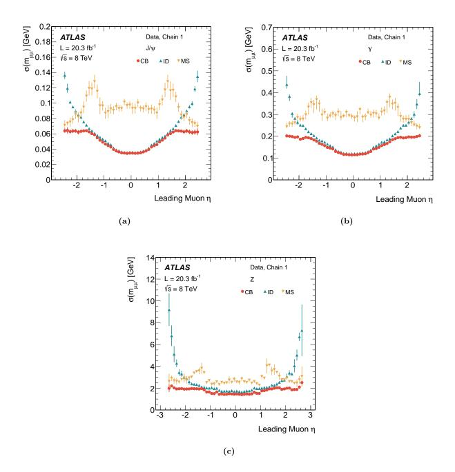
**Figure 3.9:** Invariant mass resolution  $\sigma(m_{\mu\mu})$  for ID, MS and combined measurements observed in data at  $\sqrt{s} = 8$  TeV for J/ $\psi \to \mu\mu$  (a),  $\Upsilon \to \mu\mu$  (b) and Z $\to \mu\mu$  (c) as a function of  $\eta$  of the highest  $p_T$  muon of the pair.
