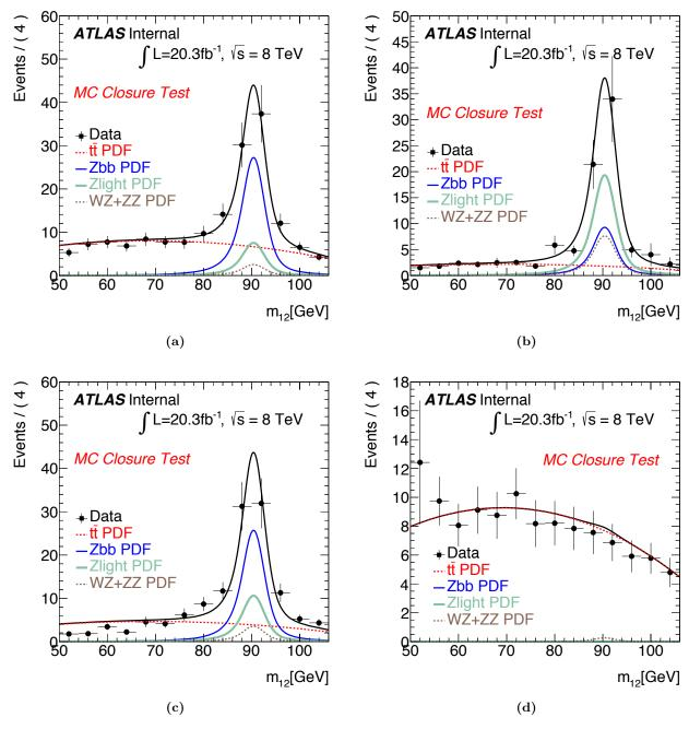
Figure 5.10: Simultaneous fit to data at  $\sqrt{s}$ =8 TeV using the  $m_{12}$  variable in the various control regions of the  $Z + \mu\mu$  analysis, namely inverted  $d_0$  significance (a), inverted isolation (b), same-sign (c) and  $e\mu + \mu\mu$  CR (d).
