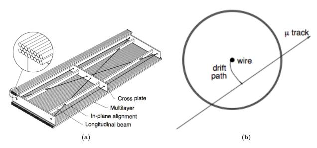
**Figure 2.19:** (a) Schematic drawing of an MDT chamber where structural components are indicated. (b) Drift tube operation in a magnetic field with curved drift path.
