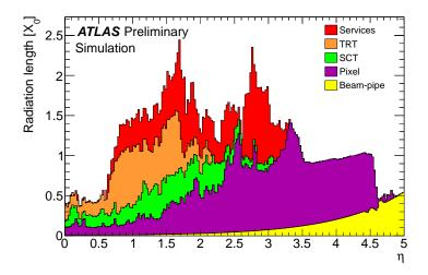
Figure 3.2: Distribution of the material in units of radiation lengths  $X_0$  traversed by electrons before reaching the calorimeter. The filled colour areas matches with contributions of different detector elements.
