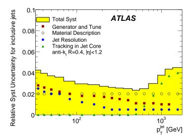
**Figure 3.11:** Relative systematic uncertainty on the jet energy scale for inclusive jets treated with the anti-kt algorithm (R=0.4) and  $|\eta|$  <1.2. The various contributions to the total uncertainty are reported as a function of  $p_T^{\text{jet}}$ .
