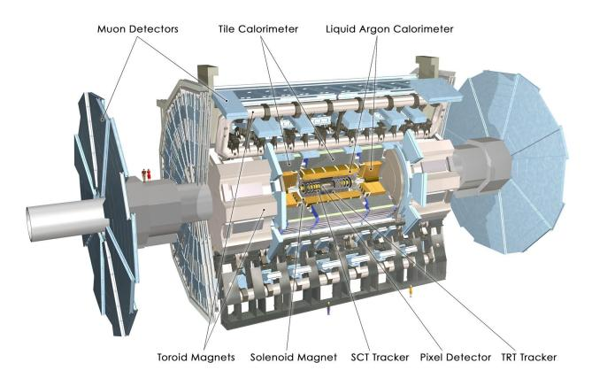
Figure 2.6: Schematic layout of the ATLAS experiment.
