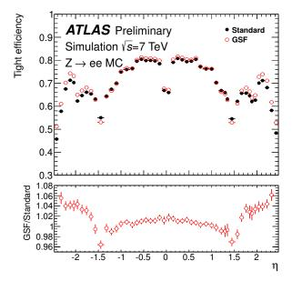
**Figure 3.5:** Electron reconstruction efficiency for a specific identification menu as a function of the pseudorapidity range for GSF (open red) and standard (solid black) electrons. The ratio of the GSF to the standard distribution is also provided in the bottom part of the plot.
