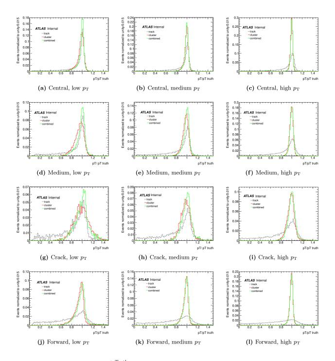
Figure 4.17: Improvement in  $p_{\rm T}/p_{\rm T}^{\rm Truth}$  for Monte Carlo single electrons after the E-p combination, as compared to the standard approach ( $E_{\rm Clus}$  only) and the track distribution as well.
