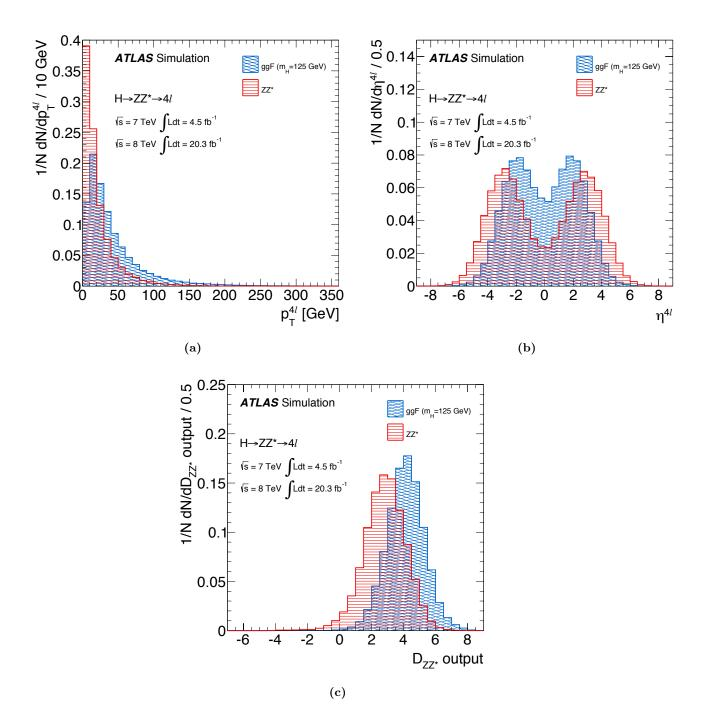
**Figure 5.6:** Input variables,  $\eta^{ZZ}$ ,  $p_T^{ZZ}$  and the KD distributions for the Higgs signal and the dominant  $q\bar{q} \to ZZ$  samples after the standard cutflow in the mass range (115<  $m_{4l}$  <130) GeV used for the training of the BDT discriminant.
