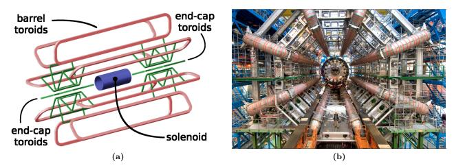
**Figure 2.7:** (a) Geometry of the coils comprising the solenoid, the barrel and end-caps toroids. (b) Frontal view of the barrel toroid operating inside the muon system.
