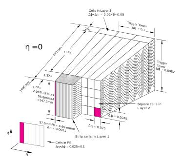
Figure 2.13: Graphic representation of the electromagnetic calorimeter and its modularity.
