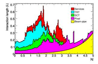
**Figure 2.11:** Material distribution described by the interaction length  $\lambda$  for hadronic interactions at the exit of the ID envelope including the services. The distribution is shown as a function of  $\eta$  and averaged over  $\phi$ . The breakdown indicates the contributions of external services and individual sub-detectors.
