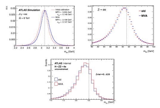
Figure 4.6: Di-electron invariant mass distributions for simulated  $J/\Psi \rightarrow ee$ ,  $Z \rightarrow ee$  and  $H \rightarrow ZZ^* \rightarrow 4e$  decays comparing the standard and the MVA calibration responses. The dashed line indicate the PDG-mass [71] of the resonances.
