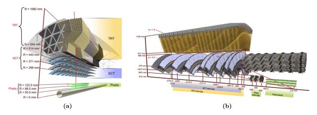
Figure 2.9: Pictorial sketch and localisation of the different modules comprised in the Inner Detector in the barrel (a) and in the end-caps (b) when traversed by a 10 GeV charged particles (red lines) for different pseudorapidity values ( $|\eta|$ =0.3, 1.4, 2.2).
