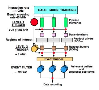
Figure 2.22: Trigger and DAQ systems developed in ATLAS
