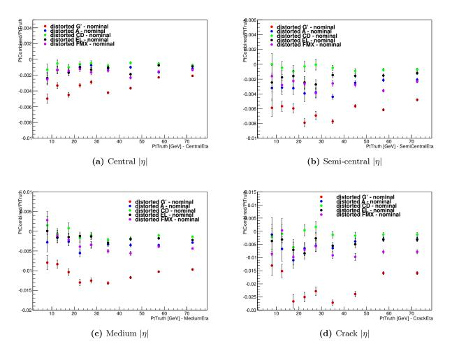
Figure 4.30: Distributions of  $(p_{\rm T}^{\rm Comb}/p_{\rm T}^{\rm Truth})_{\rm Distorted} - (p_{\rm T}^{\rm Comb}/p_{\rm T}^{\rm Truth})_{\rm Nominal}$  as a function of  $p_{\rm T}^{\rm Truth}$  in the various  $\eta$  regions. The nominal geometry response is compared with the other distorted samples.
