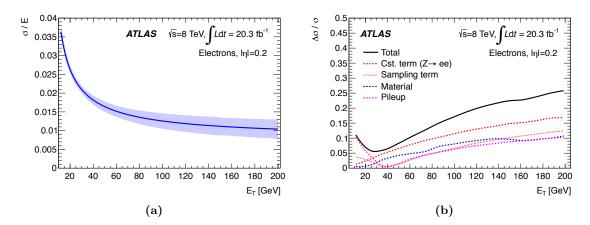
Figure 4.10: (a) - Resolution curve and its uncertainty as a function of  $E_T$  for electrons with  $|\eta| < 0.2$ . (b) -Contributions of the different uncertainties to the relative resolution uncertainty as a function of  $E_T$  for electrons with  $|\eta| < 0.2$ .
