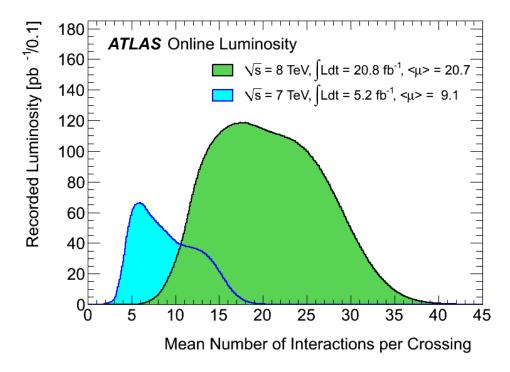
Figure 3.13: Luminosity-weighted distribution of the mean number of the interaction per crossing in data for 2012 at  $\sqrt{s}$ =8 TeV using an integrated luminosity of 20.8 fb<sup>-1</sup> and 2011 at  $\sqrt{s}$ =7 TeV for 5.2 fb<sup>-1</sup>.
