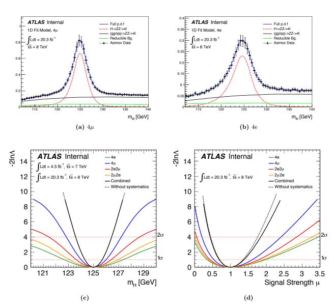
Figure 5.22: 1D fitting of signal + background model to the Asimov dataset generated for a Higgs boson at  $m_H$ =125 GeV + background in the  $4\mu$  (a) and 4e (b) categories. Likelihood scan of  $m_H$  (c) and  $\mu$  (d) for 1D fit of Asimov dataset generated at  $m_H$ =125 GeV + background ( $\sqrt{s}$ =7 TeV and  $\sqrt{s}$ =8 TeV).
