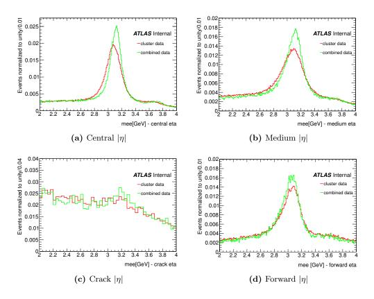
Figure 4.21: Invariant mass distributions of  $J/\Psi \to ee$  data events, with and without the combination in effect. The data used corresponds to 21 fb<sup>-1</sup> of pp collisions at  $\sqrt{s} = 8$  TeV, recorded during 2012.
