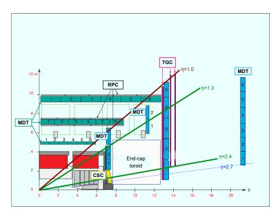
**Figure 3.7:** Schematic picture showing a quarter-section of the muon system in a plane containing the beam axis. The position of MDTs, RPCs, TGCs and CSCs is indicated in figure.
