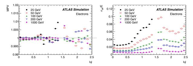
**Figure 4.5:** Most probable value (MPV) of  $\frac{E}{E_{\text{truth}}}$  and relative effective resolution  $\sigma_{\text{eff}}/E$  as a function of  $|\eta|$  for different energies.
