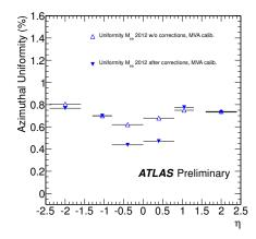
Figure 4.2: Non uniformity of the energy response of an electron candidate as a function of  $\eta$  with and without corrections.
