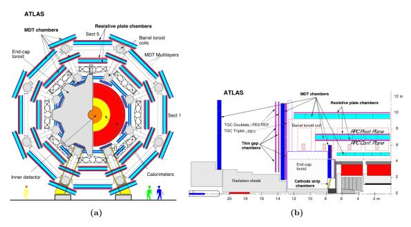
**Figure 2.18:** Schematic view of the muon spectrometer in the x-y (a) and z-y (b) projections.
