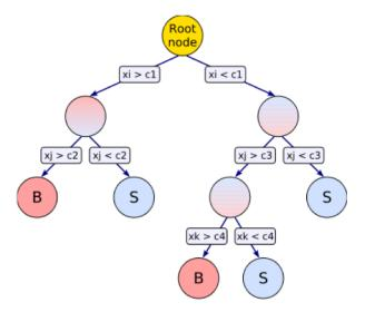
**Figure B.1:** Schematic sketch of a decision tree. Starting from the root node, a sequence of binary splits using the discriminating variables  $x_i$  is applied to the input data. Each split uses the variable that, at a given node, gives the best separation between signal and background when being cut on. The leaf nodes at the bottom end of the tree are labelled S for signal and B for background depending on the majority of events that end up in the respective nodes.
