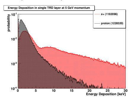
**Figure 2.10:** Histogram of energy entries in a layer of the TRT for 5 GeV particles. The proton spectrum is shown in black and the positron spectrum in red.
