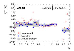
**Figure 4.7:** Ratio of average presampler energies for electrons in data and simulation as a function of pseudorapidity, before and after corrections to the first and second layer intercalibrations as well as the calibration of the presampler layer. The full lines with shaded bands represent the energy scale and its uncertainty
