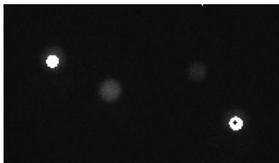
Figure 25: Centre location in a z-stack. The overlaid white circle indicate the proximity of the particle centre in the z-direction and the black dot, that the centre is located in this z plane.
