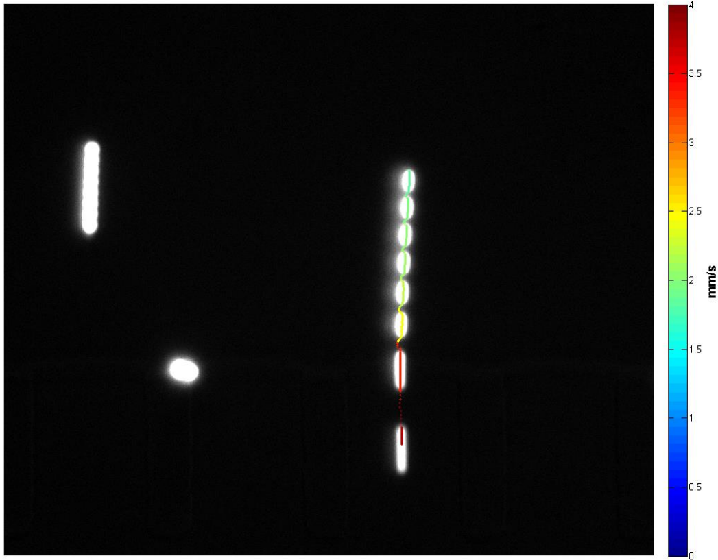
Figure 29: Velocity reconstruction along a streak trajectory using square pulse illumination
