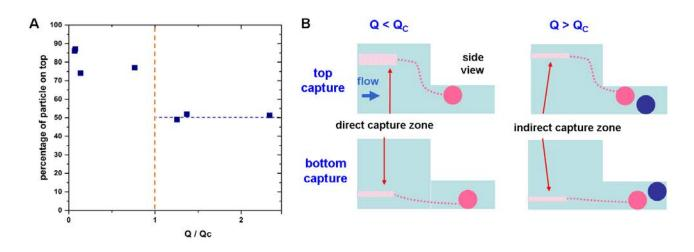
Figure 71: A-percentage of particles captured by the top wall of the pore as a function of the flow rate. B-Schemes of the main capture mode for the line (Q<Q<sub>c</sub>) and in the invasion regime (Q>Q<sub>c</sub>).
