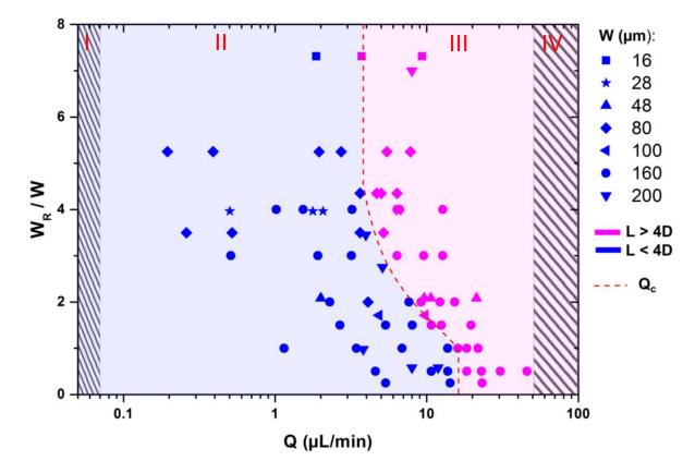
Figure 41: Phase diagram of 2d clogging for D=4 μm PMMA particles. Blue points are line type clogs (clog length L<4D, zone II). Magenta points are invasive clogs (clog length L>4D, zone III). The dashed red line is the critical flow rate Q<sub>c</sub>. Hatched zones correspond to areas of no particle deposition (zones I and IV).
