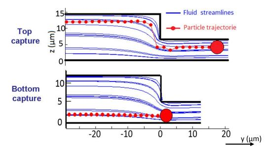
Figure 52: Trajectory of two depositing particles in the z-y plane (dotted red line) overlaid on the fluid streamlines (blue lines), one on the top wall and the other on the bottom one. The particles initially travels along a fluid streamline and cross fluid streamlines approaching the constriction. The flow rate is Q=0.6 µL/min.
