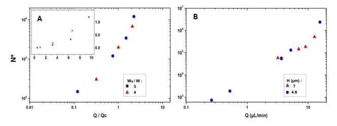
Figure 45: A- Variation of N<sup>\*</sup> with the flow rate Q, normalized by the critical flow rate QC, for two ratio of widths (W=160 $\mu$ m). Inset: N<sup>\*</sup> vs. Q for the same conditions. B- Evolution of the number of particle flowing through the pore prior to clogging with the height of the channel. We used the same experimental conditions as in the Figure 40.
