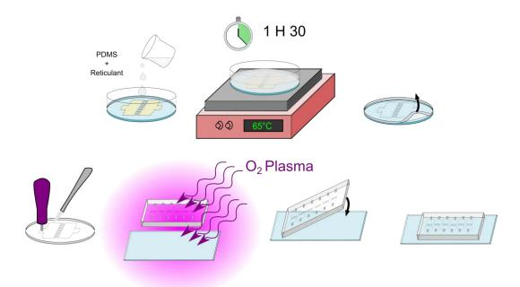
Figure 32 : Schematic illustration of the procedure of PDMS replica moulding.
