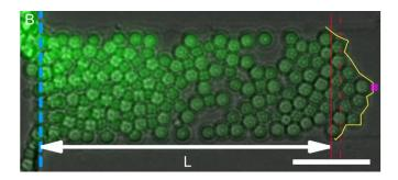
Figure 37: Clog of a W=28 µm pore by 4 µm PMMA in W=28 µm channel. Line (A) and invasion (B) morphologies. Dashed blue line is the constriction entrance. Yellow stroke defines the clog's front line. Dashed red line is the average length of the line front. Continuous Red line is the maximum density line in the clog's front line. Magenta square is the maximum penetration length. Scale bar is 20 µm.
