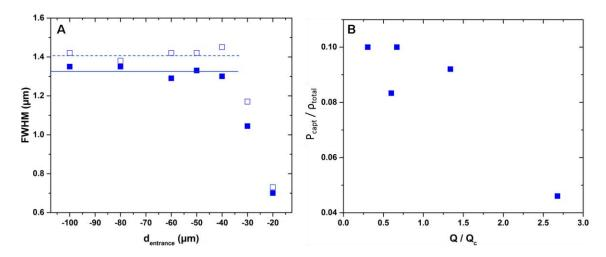
Figure 64: A- Evolution of the full width at half maximum (FWHM) of the probability density for various distances from the pore entrance, for the bottom (open symbols) and the top (plain symbols) parts. The two lines are guides for the eyes. B- Evolution with the flow rate of the ratio between the particle concentration within the capture zone and the total concentration.
