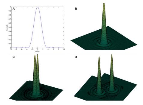
Figure 17 : A- Normalized Intensity of the Airy pattern across a diametrical section. B- Airy pattern of a single point. C-Diffraction patterns of two points not resolved by the imaging system according to Rayleigh criterion. D- Diffraction patterns of two points resolved by the imaging system.
