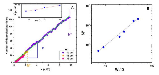
Figure 44: A- Variation of N<sub>p</sub> with N in the invasion regime for different pore widths (W=36, 48 and 80  $\mu$ m) at Q/QC = 1.5. The line is a linear fit with a slope of 1.32x10<sup>-3</sup>. Insert-Variation of P (x 10<sup>-3</sup>) with the rescaled width of the pore W/D. The line is a linear fit with a slope of 2x10<sup>-5</sup>. B-Variation of N\* with the rescaled pore width W/D. The dotted line is a quadratic fit such as N\*=1022(W/D)<sup>2</sup>.
