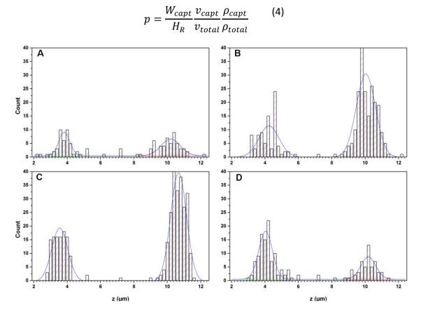
Figure 63: Repartition of particles in the z direction in the reservoir at 100 $\mu$ m from the pore entrance for Q/Qc =0.35 (A); 0.71 (B); 0.92 (C); 1.23 (D). The central zone of the reservoir (the highest speeds) is depleted in all cases. Particles are mainly in two zones centred on z=4  $\mu$ m and z= 10.5  $\mu$ m, for all flow rates.
