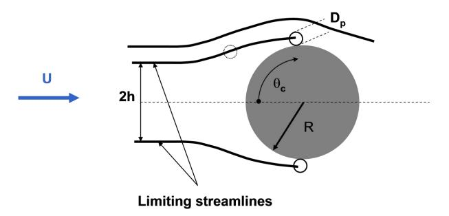
Figure 15: Capture of a particle in the interception mode. All the particles centres which lie in between the two limiting streamlines are captured by the collector (full grey circle). Outside of this zone, particles are not captured. The scheme is purposely not at the scale.
