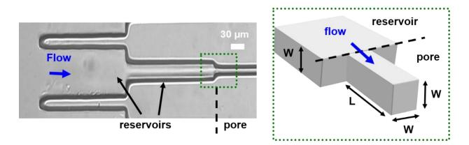
Figure 74: Scheme of the 3D geometry in top (left) and side (right) view. The blue arrows indicate the flow direction. Particles flow through two consecutives reservoirs prior entering into the pore/constriction. There is a factor of three between the width of the smaller reservoir and the pore one, and also between the larger and the smaller reservoirs.
