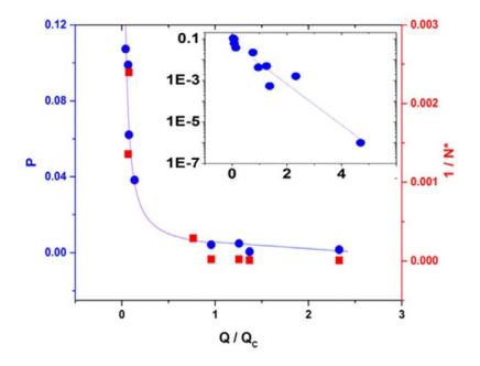
Figure 43: Variation of particle deposition probability P (circles) and  $1/N^*$  (squares) with the scaled flow rate  $Q/Q_c$ . The blue curve is an exponential fit with a decay constant equal to 0.08. Insert: P vs. flow rate in "log-lin" plot.
