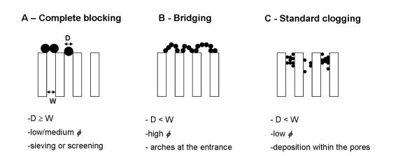
Figure 3 : Different mechanisms of clogging which depend mainly on the degree of confinement W/D and the particle volume fraction in solution  $\phi$ .
