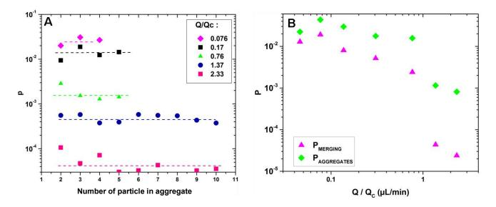
Figure 66: A-Probability of aggregate formation for various flow rates. The dashed lines correspond to the average probability for each flow rate used in B. B-Variation of the average probability to form an aggregates which size in between 2 and 10 (diamonds) and to merge two aggregates (triangles) whatever their sizes, with the flow rate.
