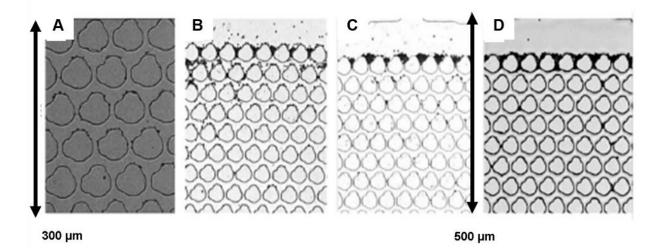
Figure 2: Images of a model porous medium in which flow a diluted colloidal suspension with the same flow velocity (60 mDarcy) (from ref. [37]). In each case, the particle size is different: 3 μm in (A), 4 μm in (B), 5 μm in (C) and 7 μm in (D).
