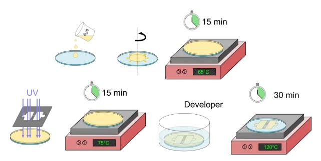
Figure 30 : Schematic illustration of the SU8 soft-lithography process
