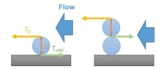
Figure 103: Hydrodynamic torque acting on a deposited particle. Left: particle deposited on the pore wall. Right: particle deposited on top of another particle.
