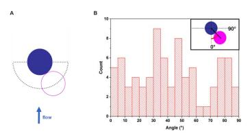
Figure 56: Doublet formation. The grey dotted semi-circle corresponds to the final different positions the flowing particle centre (hollow pink circle) when it is captured by an immobile particle (blue circle). B- Histogram of angle distribution between the two particles according to the flow direction. We do not make any distinction between the right and the left quarter, we add them in order to get only the angle variation in between 0, and 90° (insert)
