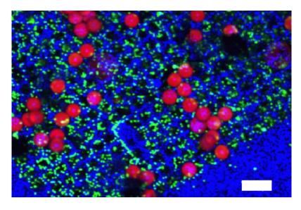
Figure 4 : Confocal image of a microsieve during fractionation of bidisperse suspension (initial volume fraction of 1 $\mu$ m (green) and 9.7  $\mu$ m (red) particles in solution are respectively 5.3 10<sup>-7</sup> and 2. 3 10<sup>-5</sup>, 30 minutes after the beginning of the experiment. The grid is in blue colour.
