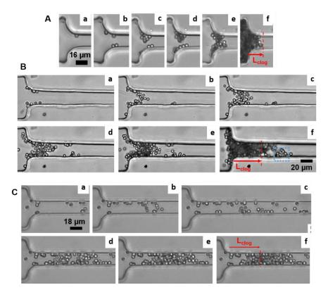
Figure 106: Successive images of clog build up. A- 4 $\mu$ m PS particles in solution of H2O/D2O in a W=16  $\mu$ m pore (cf. Figure 75). B- 4  $\mu$ m PMMA particles in a solution of 29% of sucrose in a W=24  $\mu$ m pore. C- 4  $\mu$ m PMMA particles in a solution of 64% of urea in W=18  $\mu$ m pore.
