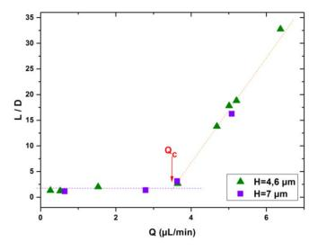
Figure 40: Variation of L/D with the flow rate Q for two different heights of the pore (H=4.6 and H=7  $\mu$ m).
