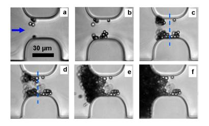
Figure 78: Images of the different construction steps of a clog in a pore with small  $L_{flat}$ =0.4W. Blue arrow on a indicates the flow direction, the dashed blue line on c and d indicates the middle of the pore. a-b: deposition of the first particles at the pore entrance within the corners. c-d growth of two aggregates on the opposite sides of the pore on the entrance half the pore. Those aggregates grow until they finally merge and clog the pore (e-f).
