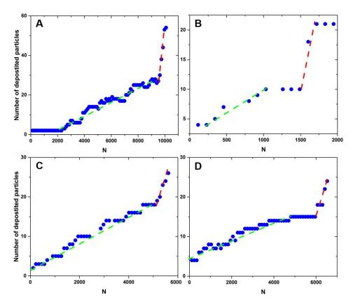
Figure 83: Evolution of the number of particles deposited in the pore for four different channels as a function of the particle flown through the pore N. Experiment is run in a W=16 $\mu$ m H=12 $\mu$ m channel with 4 $\mu$ m particles with  $\phi$ =5.10-5 and  $\Delta$ P=30mbar. Even though clogs where formed under the same flow and geometry conditions deposition curves and the clog structure are different.
