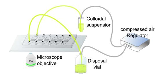
Figure 33: Experimental set-up. The colloidal suspension is injected in the microfluidic device applying a pressure drop (ΔP) between the inlet and outlet of the microchip.
