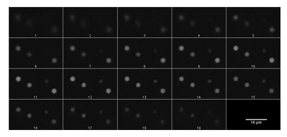
Figure 24 : Confocal z-stack of 4μm colloids (Δz=0.5 μm between 2 images).
