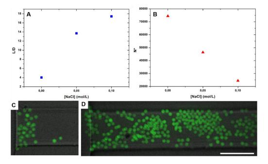
Figure 105: Influence of ionic strength on clogging at pore's scale in W=36 $\mu$ m channel at Q/Qc=1.1. A-Evolution of the clog's length with salt concentration; B- Evolution of the number of particle flowing through the channel prior to clog with salt concentration; C- Image of a clog without addition of salt; D- Image of a clog at 0.1M of NaCl. Scale bar = 20 $\mu$ m.
