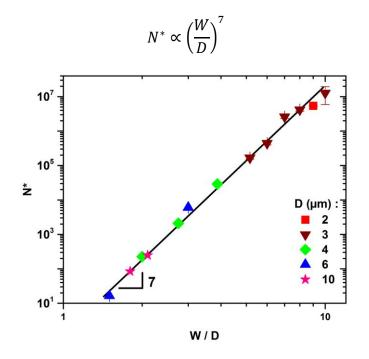
Figure 80: Evolution of the clogging efficiency with the confinement W/D. Particles are polystyrene particles of different sizes corresponding to the different symbols. The red line is a power law fit with power 7.
