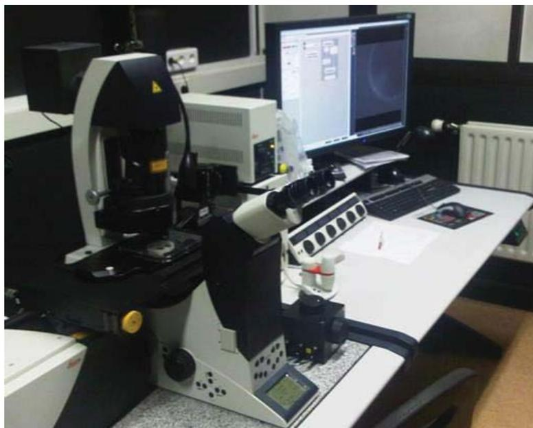
**Figure 27** Photograph of the epi-fluorescent microscope (DMI 6000B, Leica) equipped with a digital camera (DFC310 FX, Leica) used for the direct visualization of the grafted fluorescent molecule coupled with one side of the 4-CP-modified glassy carbon bead.
