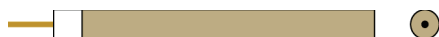
Figure II-4 Side and bottom view of the schematic representation of the commercial glassy carbon working electrodes used in routine cyclic voltammetry experiments.
