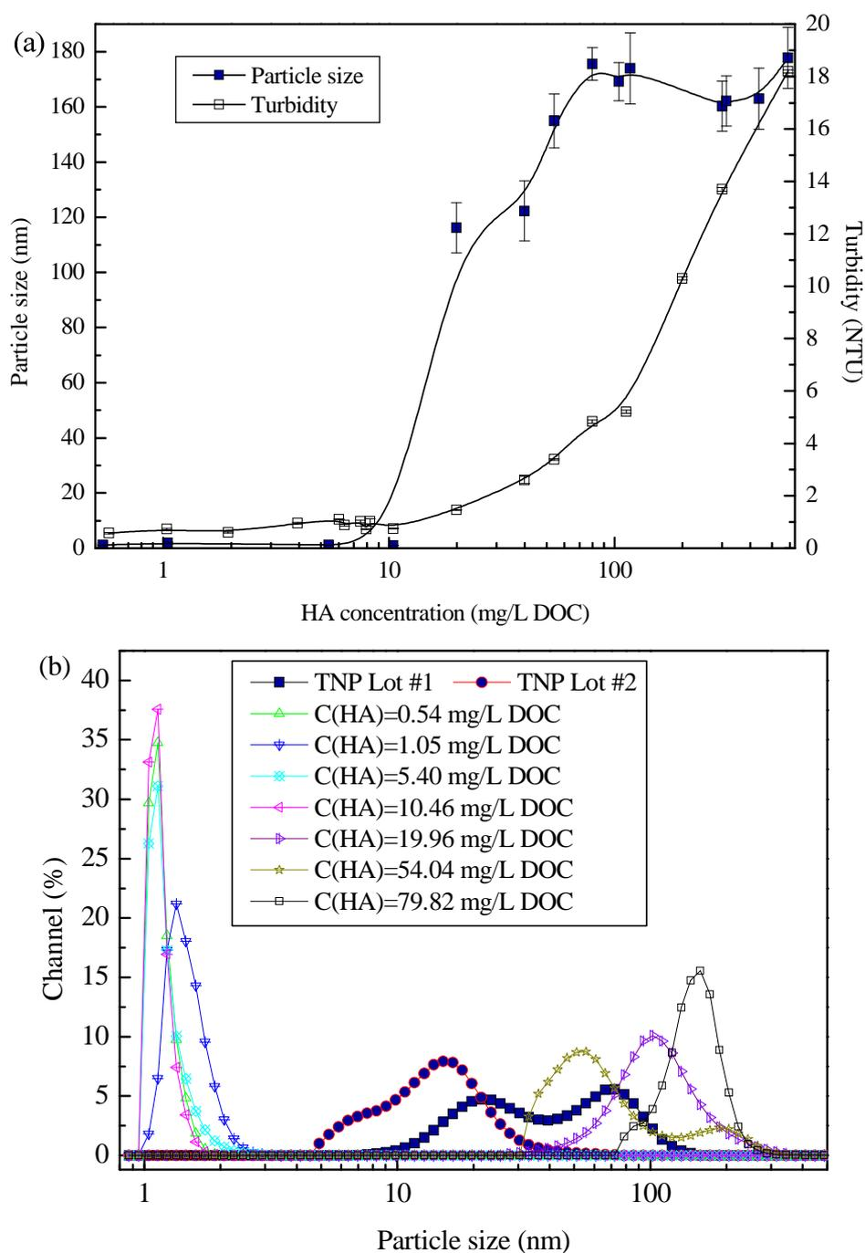
Fig. 2.10. (a) Particle size and turbidity varying with HA concentrations; (b) PSD patterns of TNPs and HA.
