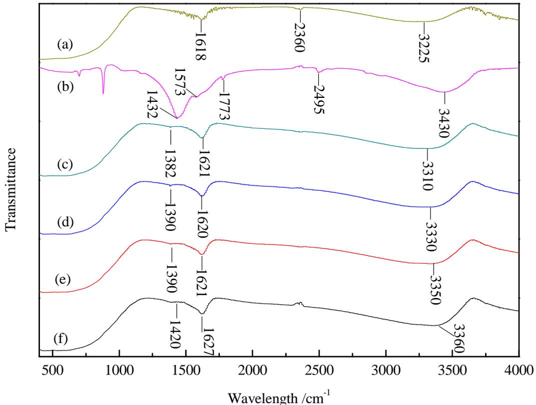
Fig. 3.6. FT-IR spectra of TNPs before and after surface modification by HA with various additive contents: (a) TNPs, (b) HA, (c) TNPs + 6.10 mg/L DOC HA, (d) TNPs + 7.06 mg/L DOC HA, (e) TNPs + 8.02 mg/L DOC HA, (f) TNPs + 9.15 mg/L DOC HA.
