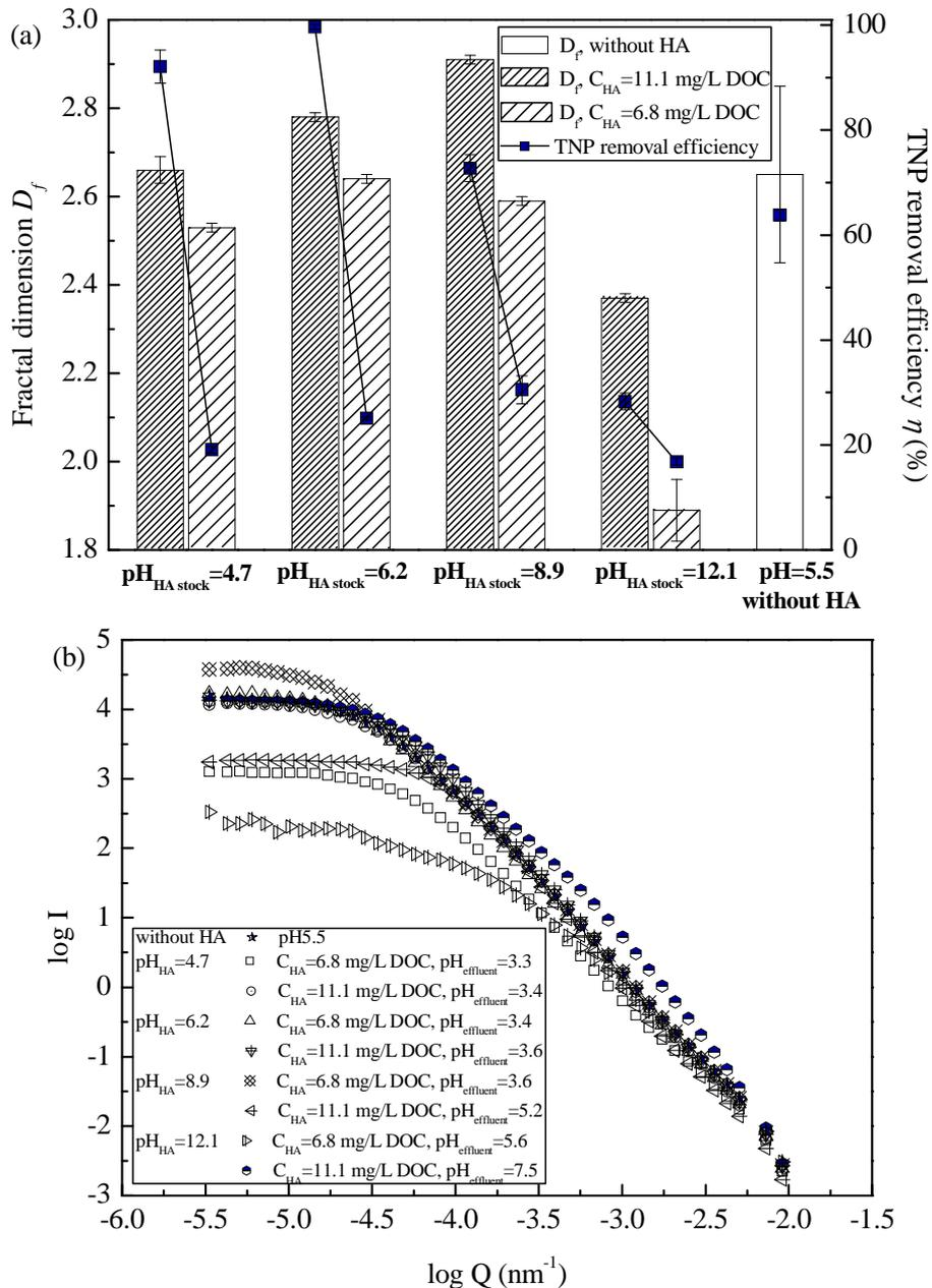
Fig. 3.24. (a) Comparison of fractal dimension values of flotation aggregates under different conditions (corresponding to Fig. 3.23); (b) Static light scattering plots of flotation flocs formed in different physiochemical conditions.
