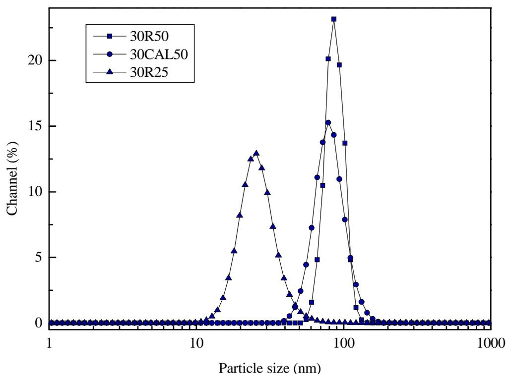
Fig. 2.12. Particle size distributions of different SNPs.
