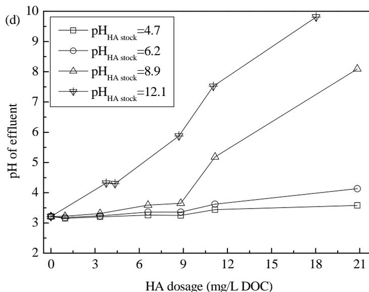
Fig. 3.18. Flotation behavior varying with HA dosage (The pH value of HA stock solution was adjusted to 4.7, 6.2, 8.9 and 12.1, respectively): (a) TNP removal efficiency, (b) HA removal, (c) zeta potential, and (d) pH of effluent.
