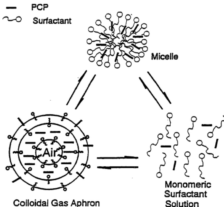
Fig. 4.18. Schematic of the solubilization process in the presence of CGAs and micelles (PCP: Pentachlorophenol, the separating target; surfactant: sodium dodecylbenzene sulfonate, hexadecyltrimethylammonium, or tergitol) (Chaphalkar, 1994).
