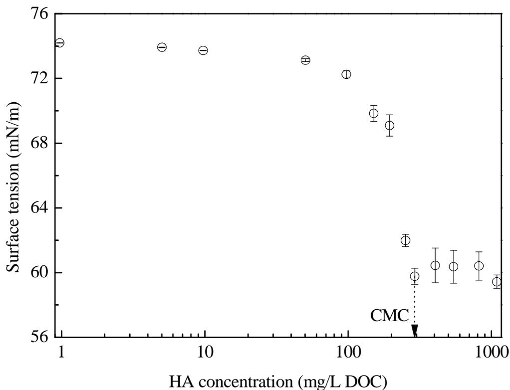
Fig. 2.9. Determination of CMC by surface tension measurement.
