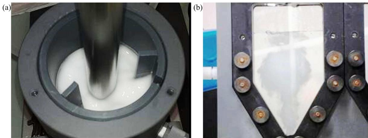
Fig. 4.3. Photos of CGA suspension (a) in the generation process, (b) after being injected into the measuring chamber from the bottom entrance.
