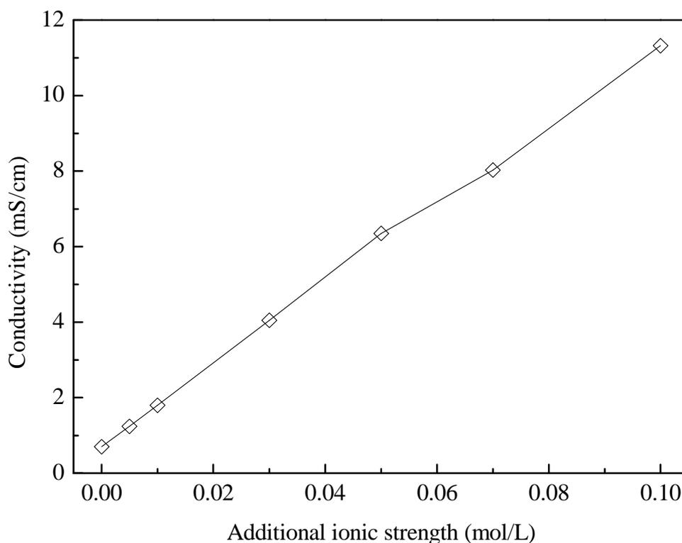
Fig. 2.5. Conductivity of TNP suspension varying with different additional IS.
