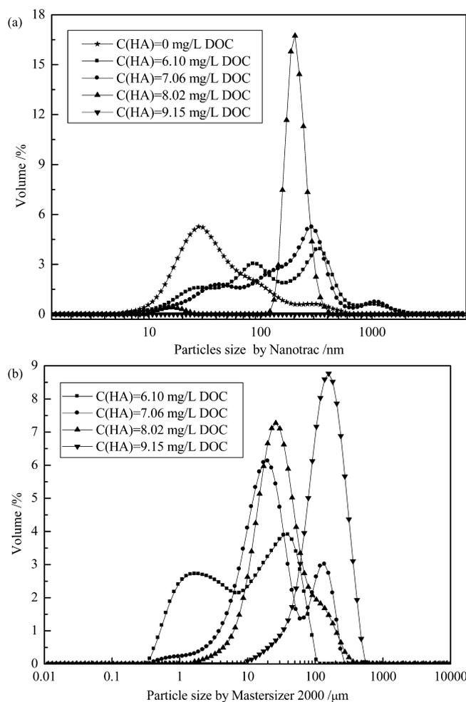
Fig. 9. Particles size distribution of surface modified TNP suspensions: (a) supernatant by Nanotracs; (b) precipitates/flocs by Mastersizer 2000.
