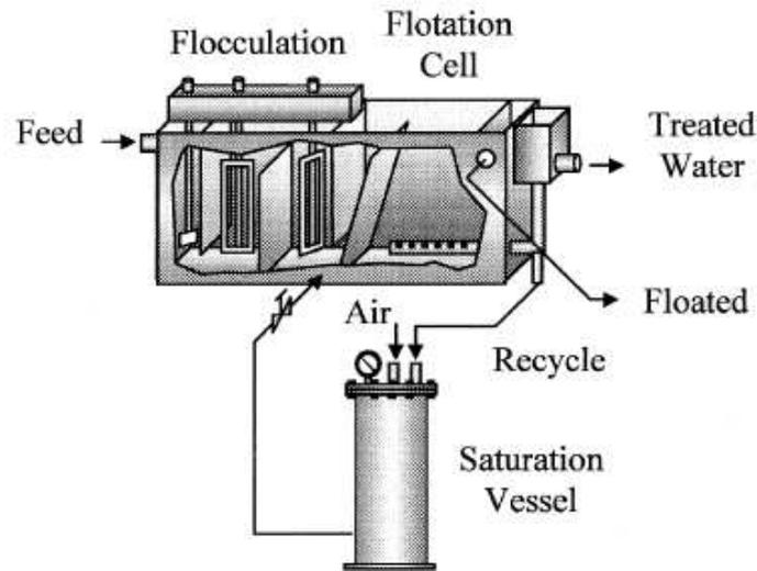
Fig. 1.6. The conventional DAF unit, with water recycle to the saturator (Rubio et al., 2002).
