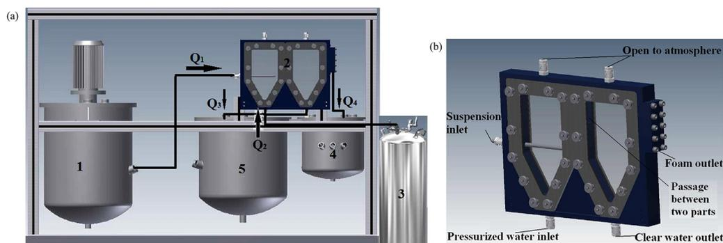
**Fig. 4.** Schematic representation of the laboratory scale continuous DAF device: (a) overview of the whole DAF system, (1). Feed tank (40 L), (2) Flotation cell ( $200 \times 105 \times 18$  mm<sup>3</sup>), (3) Saturation tank with pressurized water (20 L, the maximum tolerated pressure is 7 bars), (4) Tank for foam (5 L), (5) Tank for clean water (20 L); (b) archetype of the flotation cell.
