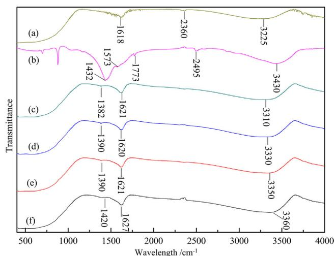
**Fig. 10.** FT-IR spectrum of TNPs before and after surface modification by HA with various additive contents: (a) TNPs, (b) HA, (c) TNPs + 6.10 mg/L DOC HA, (d) TNPs + 7.06 mg/L DOC HA, (e) TNPs + 8.02 mg/L DOC HA, (f) TNPs + 9.15 mg/L DOC HA.
