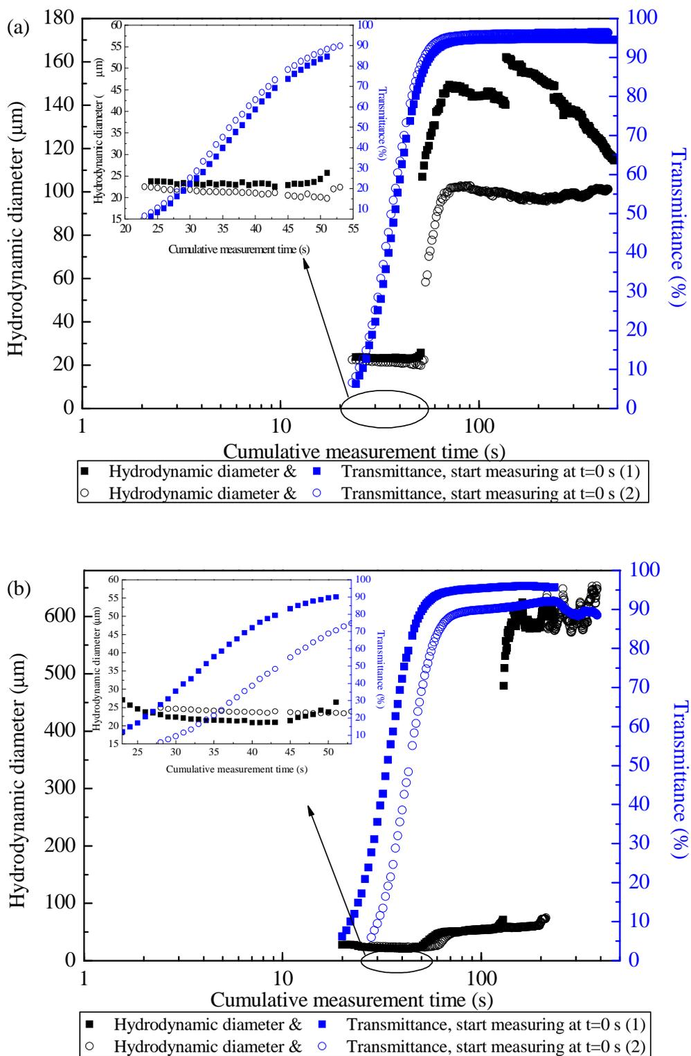
Fig. 4.12. Spraytec measurement immediately after the measurement began: (a) CTAB-CGAs; (b) SDS-CGAs. (Experiments were replicated.)
