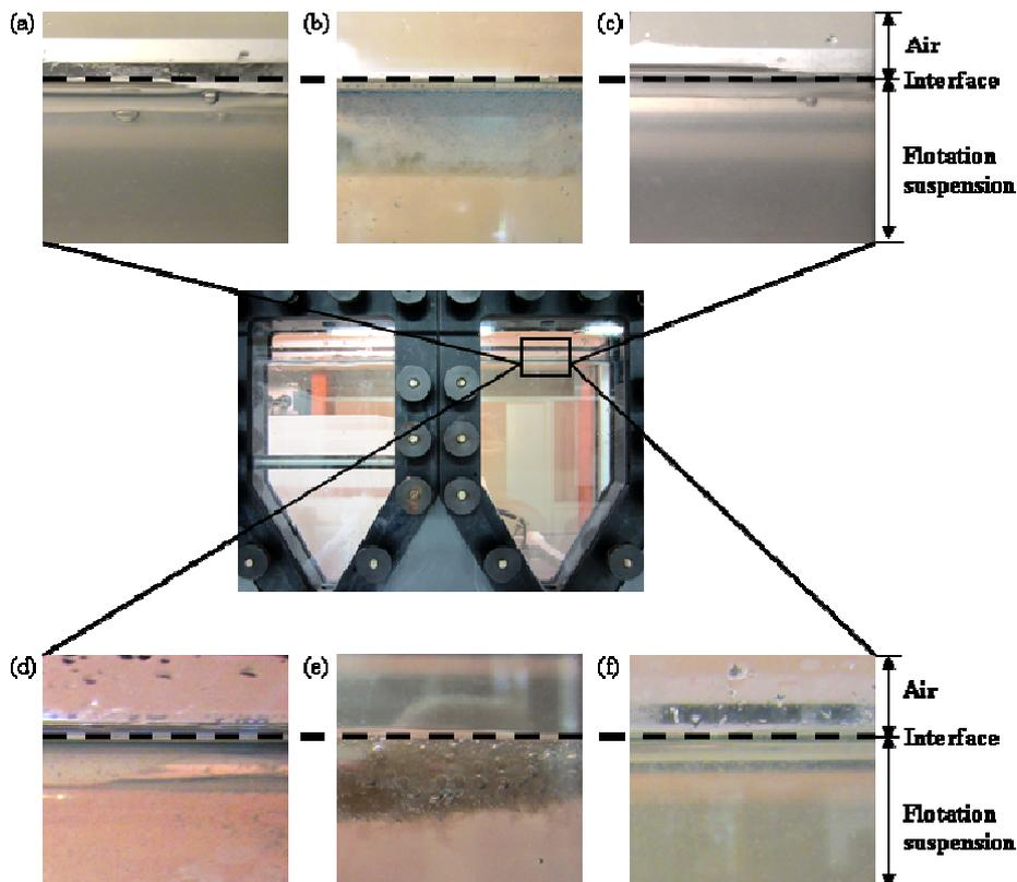
Fig. 3.21. Representative photos of the contact zone under the operating condition of  $Q_1=70$  mL/min,  $Q_2=100$  mL/min,  $Q_3=60$  mL/min, at different pH values, (a) pH=4.6, (b) pH=5.9, (c) pH=8.8, at different HA concentrations, below (d), around (e), and above (f) the optimum concentration.
