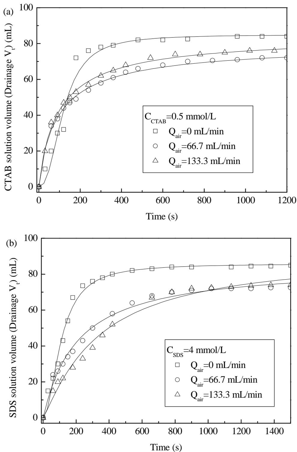
Fig. 4.8. Comparison between experimental data (scatters) and fitting drainage curves (curve) at different air flow rates: (a) CTAB-CGAs, (b) SDS-CGAs.
