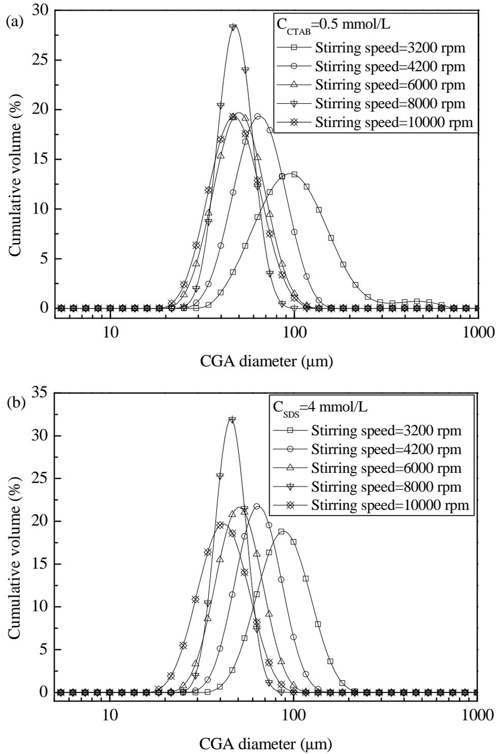
Fig. 4.15. Bubble size distribution of CGAs under different stirring speeds.
