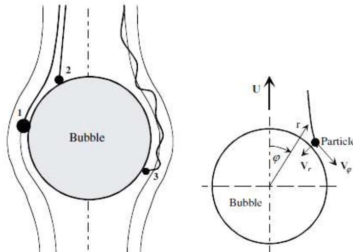
Fig. 1.5. Schematics of the (1) interception (2) gravity (3) Brownian transport mechanisms for fine particles towards a rising bubble in a rotationally symmetrical coordinate system  $(r, \theta)$ . The thick lines describe the particle trajectory while the thin lines describe the liquid streamlines (A. V. Nguyen et al., 2006).
