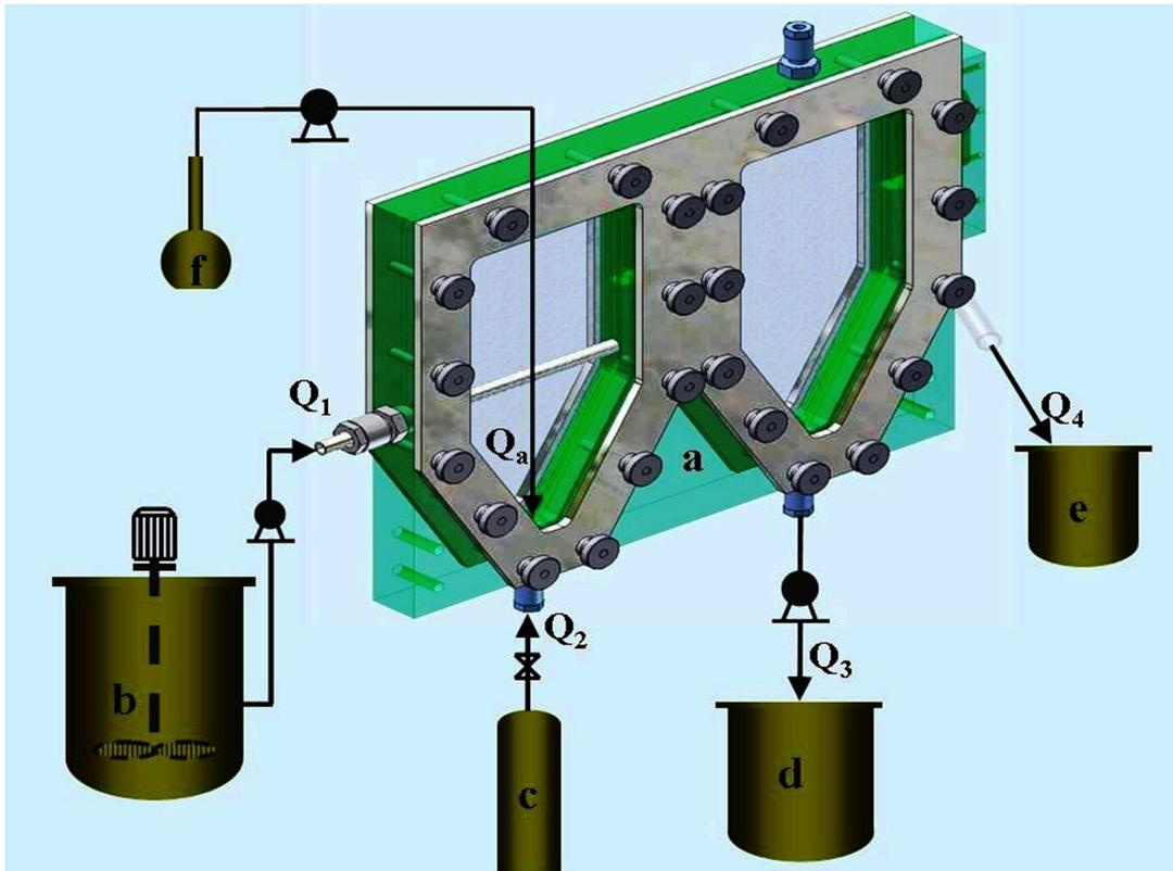
Fig. 3.12. Schematic representation of the laboratory scale continuous DAF device: (a) Flotation cell ( $200 \times 105 \times 18 \text{ mm}^3$ ), (b). Feed tank (40 L), (c) Saturation tank with pressurized water (20 L, the maximum tolerated pressure is 7 bars), (d) Tank for clean water (20 L), (e) Tank for foam (5 L), (f) Flask for the additive solution (500 mL).
