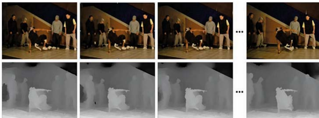
Figure 2.15: Multiview video-plus-depth: N views and corresponding depth maps from [Cagnazzo et al., 2013]
