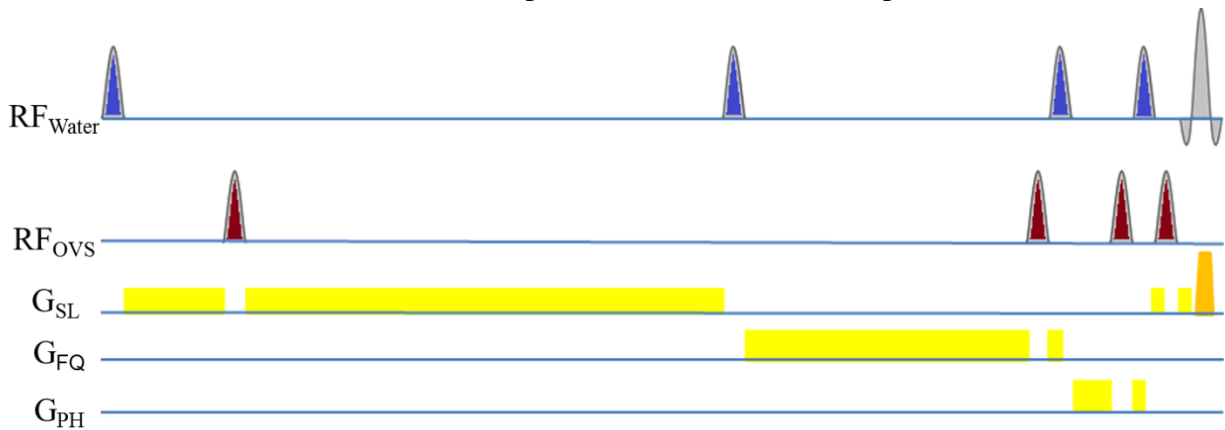
Figure 5.5. Chronogram showing the WS and OVS modules incorporated prior to the FLASH and 2D CSI sequences. The WS (blue), OVS (dark red) and excitation (gray) RF pulses were managed independently and each could use a different static B_1 -shim configuration. The spacing between consecutive pulses were 401, 355, 172, 57, 49, 26, 18 and 10 ms. For clarity, the WS and OVS modules are displayed on two separate lines. Spoiler gradients are schematically presented in yellow and slice-selection gradient in orange.
