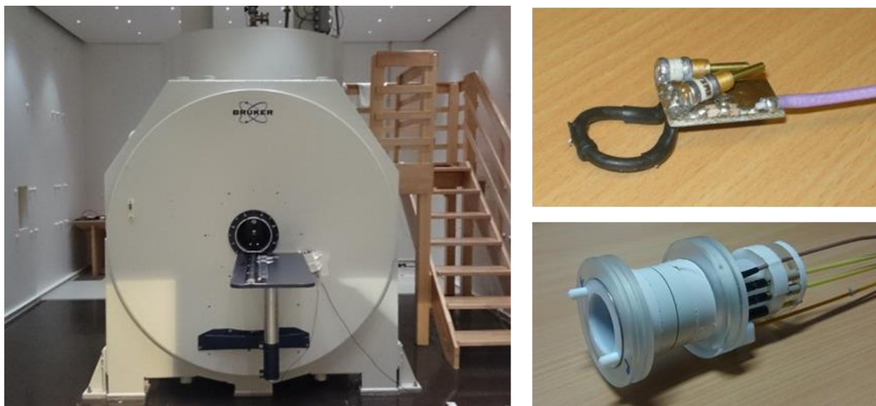
Figure 3.2. 17.2 T Bruker Biospec scanner and surface and volume coils used during the ^1\text{H} MRS study.
