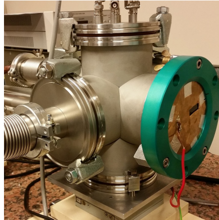
FIGURE 4.2 – Photo du cryostat.
