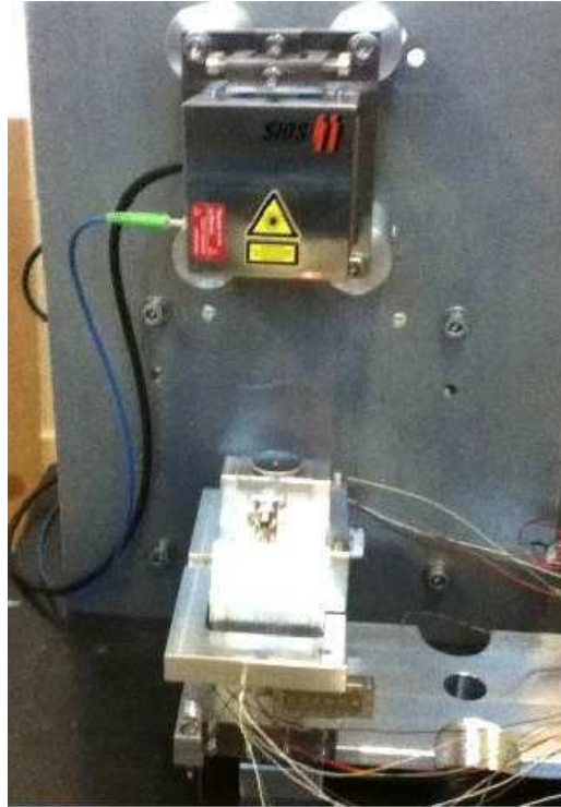
(a) Picture of SIOS interferometer used to test the movers. Precision is better than 1 nm.
