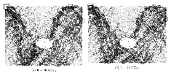
Figure E.6: Simulation of clumps  $\alpha = 0.5$  without friction at the pipe boundary. Shear localisation maps
