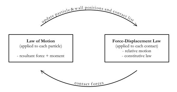
Figure 1.12: Typical time step in DEM (modified after (PFC<sup>2D</sup> Manual, 2004))
