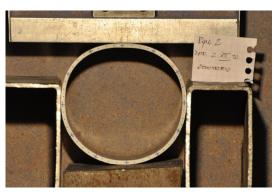
(b) PVC pipe during oedometric compression. The specimen in the experiment had 48 marks on the front face, as well as a speckle pattern, to facilitate the correlation performance
