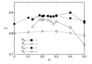
Fig. 4. Solid fraction  $\xi$  of the samples under isotropic loading versus  $\alpha$ . Error bars correspond to standard deviation calculated using of four samples. The round and square symbols represent samples made of clumps and polygons, respectively. The black and white symbols represent dense and loose samples, respectively. This convention will be maintained hereafter.
