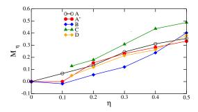
Fig. 5: (Colour on-line) Friction mobilization in the steady state as a function of  $\eta$  for different particle shapes.
