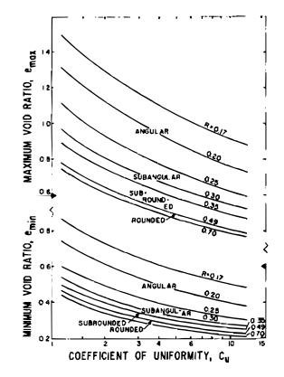
Figure 1.3: Relationship between particle roundness, sample coefficient of uniformity and extreme values of density for various sands, after (Youd, 1973)
