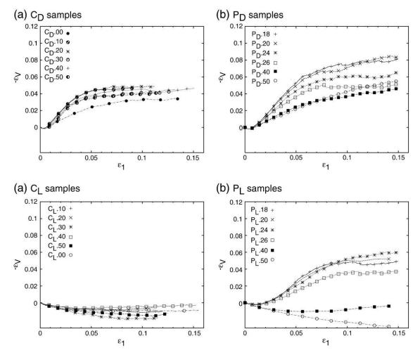
Fig. 9. Volumetric changes (computed in 2D corresponding to the area) during vertical compression for loose and dense samples made of clumps and of polygons. Positive  $-\varepsilon_v$  implies an increase of the sample volume.
