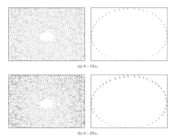
Figure D.1: Wooden grains with a PVC pipe, displacement fields. The longest arrow of particle displacement is equal to 58mm; The biggest displacement of a point on a pipe is equal to 26mm
