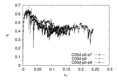
Figure 3.43: Comparison of the macroscopic results of numerical biaxial compression with clump  $\alpha = 0.5$  samples including pipes of different stiffness: 20e7Pa, 20e8Pa and 20e9Pa
