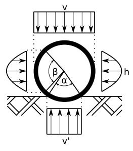
Figure 3.3: Distribution of loads acting on the pipe in Iowa method (Spangler and Shafer, 1941). The pipe is located on top of residual soil where  $\alpha$  describes the bedding angle and buried under backfill soil
