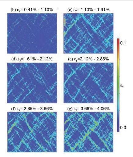
Figure 3.40: Shear strain during a vertical compression of PVC Schneebeli material in  $1\gamma 2\epsilon$ . The DIC code Photowarp revealed shear localisation zones similar to the ones obtained by us with the PVC pipe inside. Image reproduced from (Viggiani and Hall, 2008), courtesy of Viggiani and Hall
