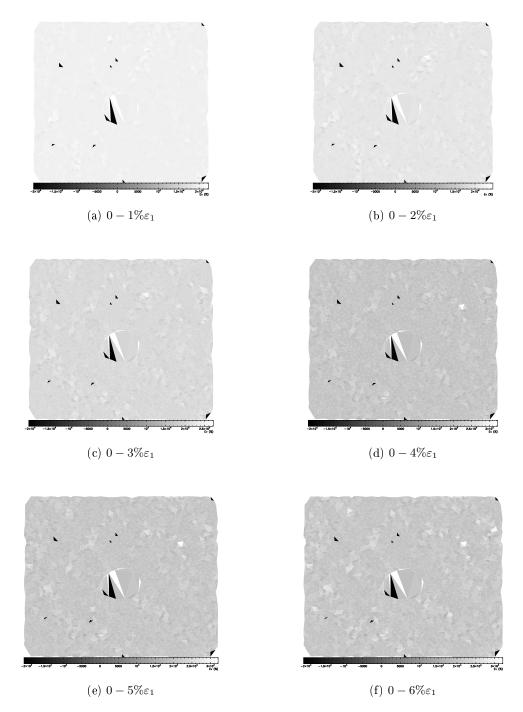
Figure D.7: Wooden grains with a PVC pipe, volumetric strain
