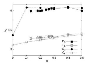
**Fig. 6.** Coordination number  $z^*$  values vs.  $\alpha$  under isotropic loading. The round and square symbols represent samples made of clumps and polygons, respectively. The black and white symbols represent dense and loose samples, respectively.
