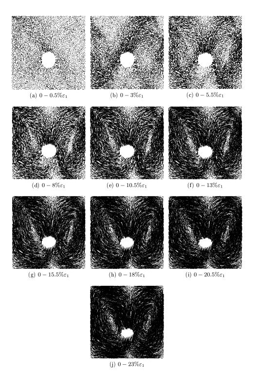
Figure 3.54: Displacement fields reduced by mean field of displacement. Clump sample with  $\alpha = 0.5$  and friction at the boundary of the pipe
