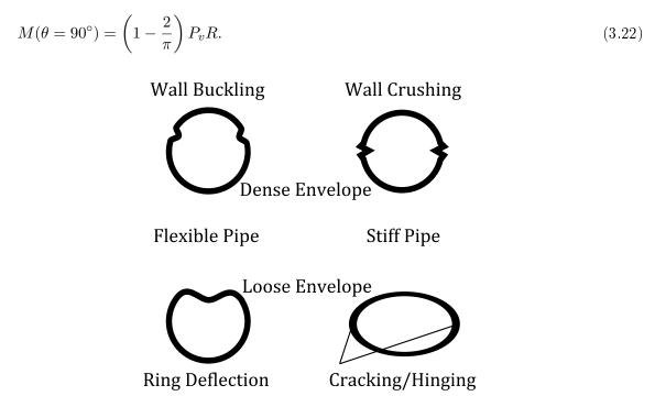
Figure 3.4: Failure modes in underground pipes (modified after (Watkins et al., 1980))
