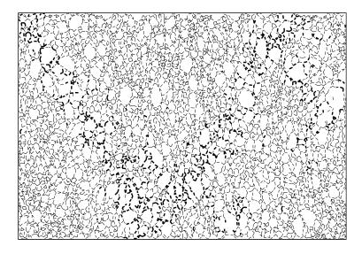
Figure 2.11: Rolling and sliding contacts in the sample of  $\alpha = 0.3$  dense clumps between 13 and  $13.5\%\varepsilon_1$ . Each persisting contact is denoted with a line connecting the discs in contact. The rolling with sliding contacts are denoted with a bold line
