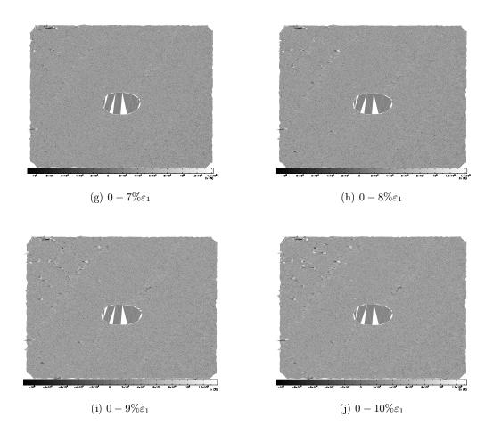
Figure D.8: PVC grains with a PVC pipe, volumetric strain
