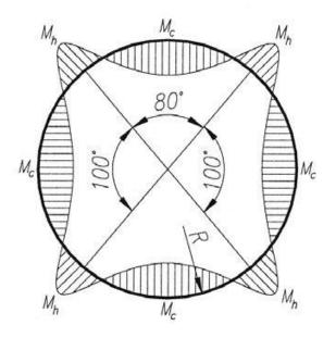
Figure 3.5: Bending moment diagram given by Spangler (after (Kunecki, 2006))
