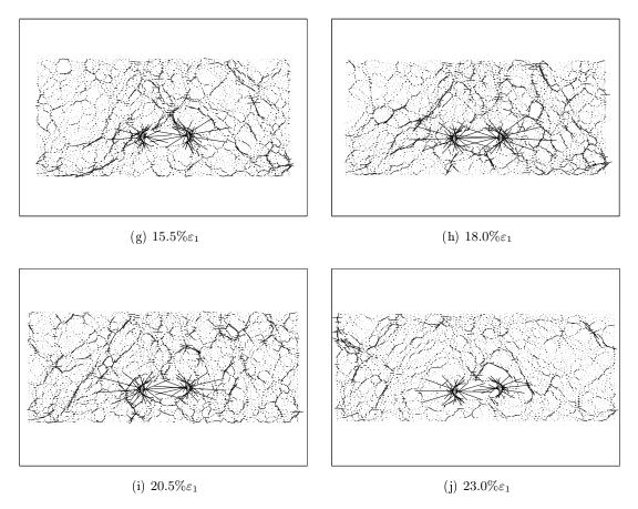
Figure E.9: Direction of particle stress. Clumps  $\alpha = 0.5$  without friction at the pipe boundary
