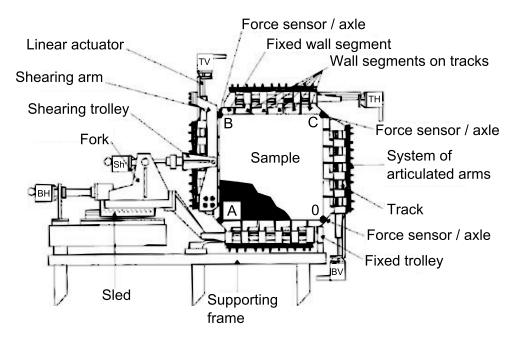
Figure 3.21:  $1\gamma 2\varepsilon$  apparatus
