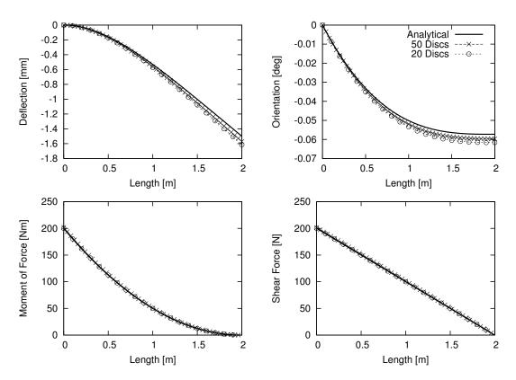
Figure 3.10: Results of cantilever beam loaded with uniform load compared with the analytical solutions
