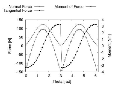
Figure 3.14: Forces in the parallel bonds representing internal forces in the elastic pipe under a single force F=250N acting on the top
