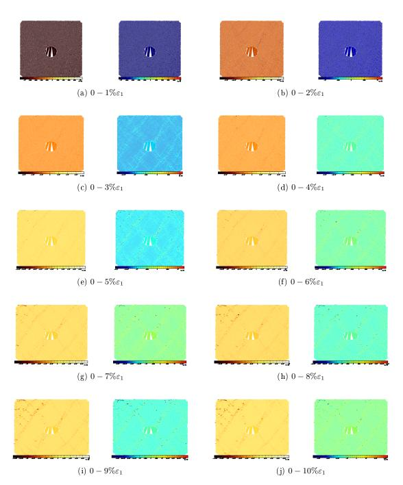
Figure D.10: PVC grains with a PVC pipe, horizontal (left) and vertical (right) strains
