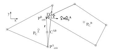
Figure A.5: Geometrical interpretation of the Shadow Overlap contact positioning phase. After finishing the previous phase it is certain that the two particles are in contact and it is particle B intruding A. The current critical corners and  $\hat{s}$  are presented. The middle of a critical corner vector  $C^{AB}$  is presented. The intermediate steps are not presented, but the final position of the first and only contact point  $D^1$  is marked
