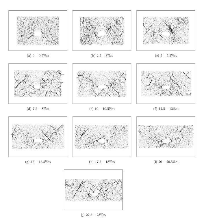
Figure 3.63: Direction of particle stress increment during biaxial compression of a clump sample with  $\alpha = 0.5$  and frictionless pipe
