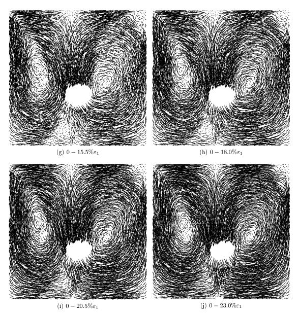
Figure E.4: Displacement fields reduced by mean field of displacement. Clumps  $\alpha = 0.5$  without friction at the pipe boundary
