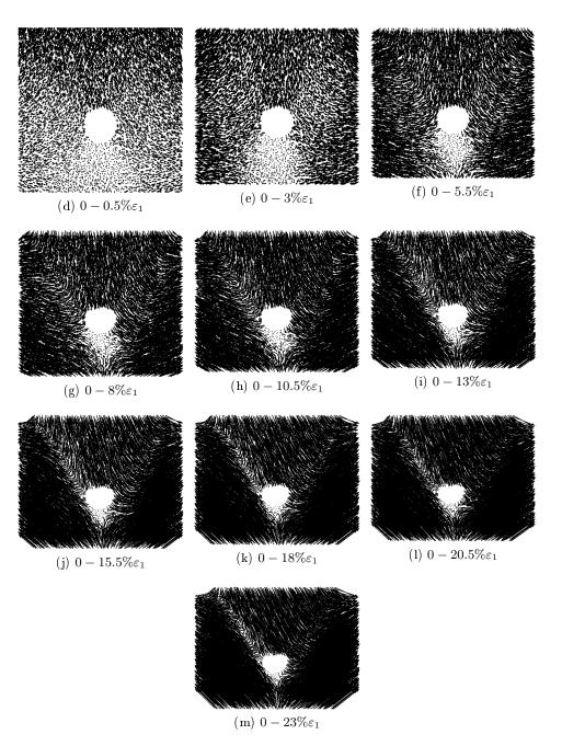
Figure 3.52: Displacement fields of a clump sample with  $\alpha = 0.5$  and friction at the boundary of the pipe
