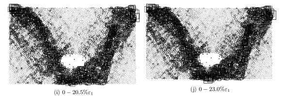
Figure E.5: Shear localisation maps. Clumps  $\alpha = 0.5$  with friction at the pipe boundary
