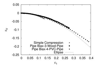
Figure 3.32: Comparison of the volumetric strains between experiments on an elastic pipe with theoretical behaviour of an ellipse. The vertical strains  $\varepsilon_1$  are not the strains of the experimental apparatus but the strains of the pipe
