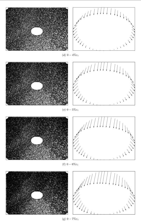
Figure D.2: PVC grains with a PVC pipe, displacement fields
