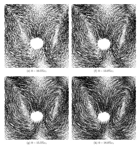
Figure E.3: Displacement fields reduced by mean field of displacement. Clumps  $\alpha = 0.5$  with friction at the pipe boundary
