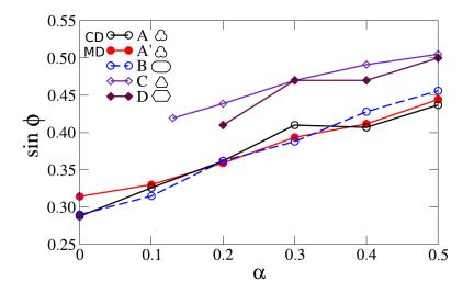
Figure 2.4: Macroscopic friction angle at the threshold of samples consisting of 5000 particles subjected to biaxial compression (CEGEO et al., 2012)
