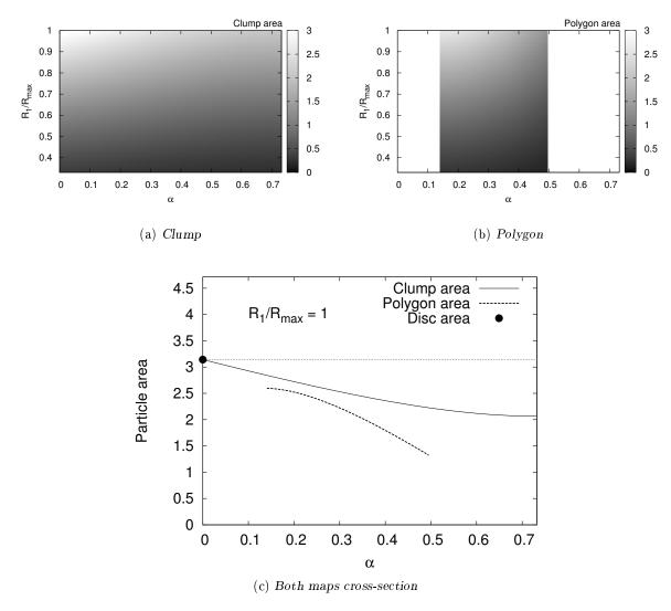
Figure B.3: Particle area functions: surface maps and a cross-section for one particular radius. The colour scale is denoting the dimensionless area in function of the shape parameter  $\alpha$  and the normalised outer radius of the particle  $R_1[-]$ . The plots are limited by the extreme values of the  $\alpha$  parameter
