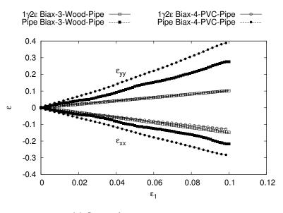
(a) Strain of the sample and pipe
