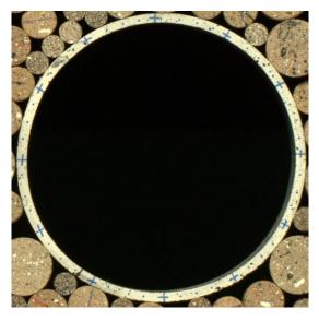
Figure 3.24: Elastic pipe surrounded by wooden grains at the beginning of a vertical compression with constant lateral pressure. The contrast of the front face of the pipe was increased by spraying fine black speckles over a white background and marking 48 points and crosses
