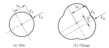
Figure 1.8: Forces acting on the grain are causing moment of force with respect to the mass centre of the particle. In case of disc the axis of normal forces is going through the grain centre, which is usually not the case in clump
