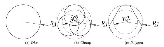
Figure 2.1: Definition of the shape parameter  $\alpha$ . Particles (b) and (c) based on the same circles have the same  $\alpha = 0.30$  but different shape
