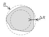
Fig. 1: An arbitrary particle shape represented by a concentric pair of circumscribing and inscribed circles.
