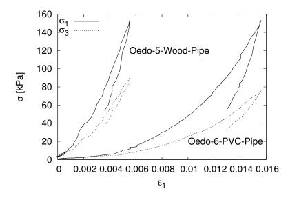
Figure 3.28:  $1\gamma 2\epsilon$  oedometric compression results of tests Oedo-5-Wood-Pipe and Oedo-6-PVC-Pipe consisting of two types of materials with a circular, elastic pipe inside. Elastic modulus of the wooden sample is equal  $28 \cdot 10^6 Pa$  while for the PVC sample it is equal to  $10 \cdot 10^6 Pa$
