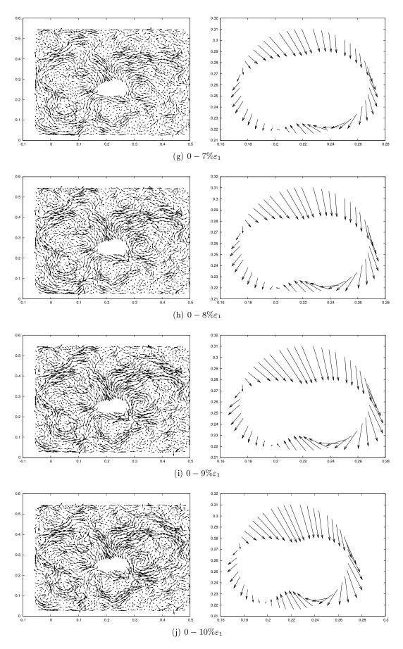
Figure D.3: Wooden grains with a PVC pipe, mean field of displacement subtracted from the displacement field  $$151\end{tabular}$
