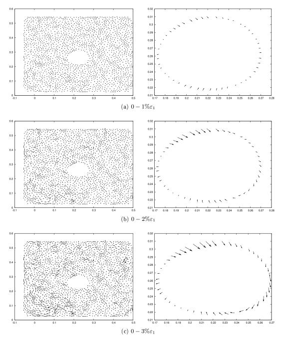
Figure D.3: Wooden grains with a PVC pipe, mean field of displacement subtracted from the displacement field. The longest arrow of displacement in the figures correspond to 4cm
