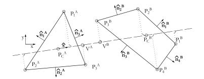
Figure A.2: Geometrical interpretation of the Shadow Overlap predetection phase together with the description of the variables used. Clearly, the difference of the projection of extreme points  $V^A - V^B$  is less than null and the particles are not in contact
