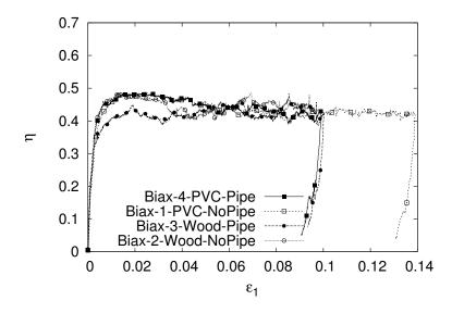
Figure 3.42:  $1\gamma 2\epsilon$  experiment results of two types of materials with or without a circular, elastic pipe inside
