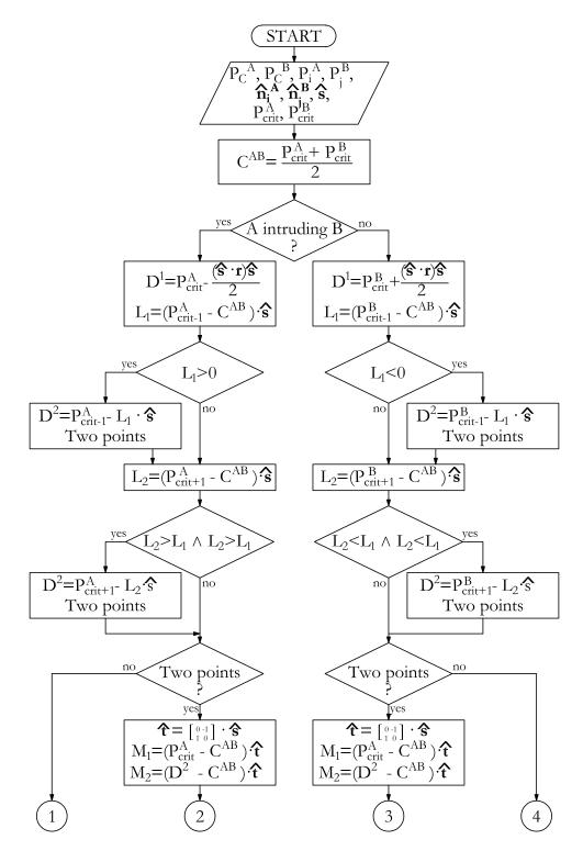
Figure A.9: Flowchart of the contact placing in Shadow Overlap method. The flowchart continues on the next page
