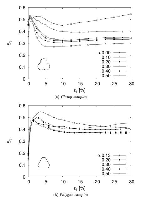
Figure 2.9: Evolution of the shear localisation indicator throughout a vertical compression test. The curves represent a mean of four samples consisting of grains of the same type
