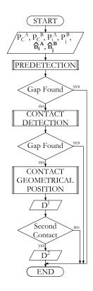
Figure A.1: Flowchart of the Shadow Overlap contact detection method for a single pair of polygonal grains A and B. This algorithm is applied to each record in the neighbour list and can be finished before the end whenever a gap is found
