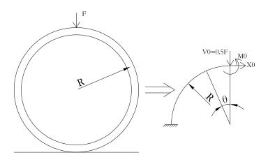
Figure C.1: Pipe quadrant modelled as a cantilever beam. The beam is fixed on one end and the other end is loaded with half of the external load acting vertically, a bending moment which correspond to internal forces and a horizontal force
