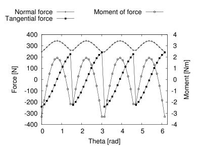
Figure 3.18: Internal forces in an elastic pipe under a single force F=500N acting on the top with horizontal displacements blocked
