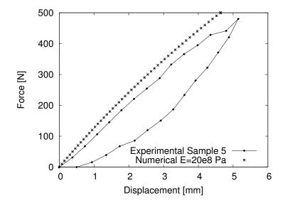
Figure 3.19: Force-displacement curve of a circular pipe oedometric compression. Comparison between experimental and numerical results
