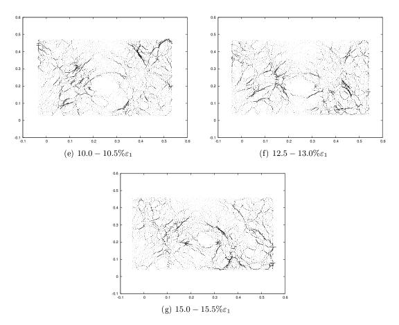
Figure E.11: Simulation of soft pipe E = 20e7Pa with clumps  $\alpha = 0.5$  and no friction at the pipe boundary. Direction of particle stress increment
