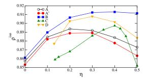
Fig. 6: (Colour on-line) Packing fraction in the isotropic state as a function of  $\eta$  for different particle shapes.
