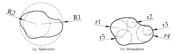
Figure 1.1: Measurements of sphericity and roundness parameters for an exemplary grain. In this case the sphericity is equal to 0.62 while the roundness is equal to 0.51
