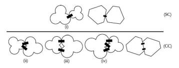
Fig. 10. Contact types for clumps and polygons: simple contacts (SC) and complex contacts (CC).
