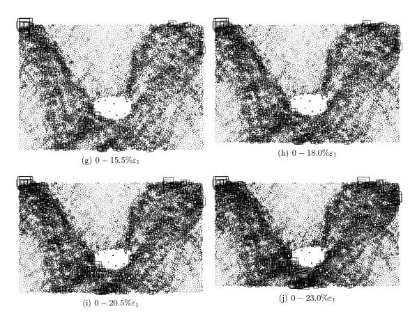
Figure E.6: Shear localisation maps. Clumps  $\alpha = 0.5$  without friction at the pipe boundary
