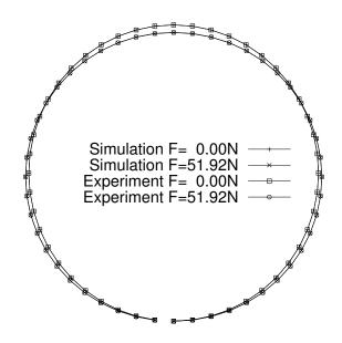
Figure 3.16: Pipe shape in the experiment and in DEM simulation in initial and final shape. Each point correspond to mass centre of a disc or to a point on the front face of the pipe
