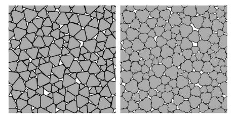
Fig. 3. Fragments of two confined dense samples with  $\alpha$  = 0.3. Sample P<sub>D</sub>.30 on the left and C<sub>D</sub>.30 on the right.
