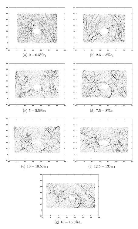
Figure 3.64: Direction of particle stress increment during biaxial compression of a clump sample with  $\alpha = 0.5$  and frictionless pipe with Young's modulus E = 20e7Pa
