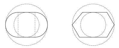
Figure 2.2: Other particle shapes used in CEGEO research program: clump made of two discs connected with a rectangle (left) and elongated polygon (right). The shape parameter  $\alpha$  of these particles is equal to 0.40
