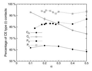
**Fig. 5.** Corner-to-edge contacts ((CE) see Fig. 2(b)) percentage in the isotropic state,  $\varepsilon_i$ . Comparison between clumps and polygons.
