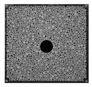
Figure 3.26: Initial position of the points used in the digital image correlation. In this case the points were placed in the centre of each particle, in the corners of the experimental apparatus and around the perimeter of the pipe
