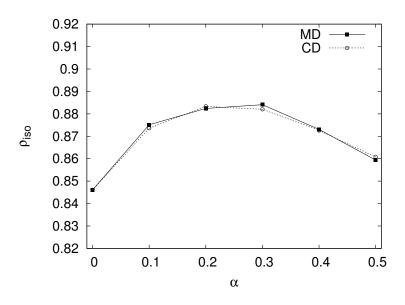
Figure 2.5: Evolution of solid fraction in the isotropic state with changing sphericity of clump grains. Comparison of numerical assemblies created in Contact Dynamics and Molecular Dynamics methods
