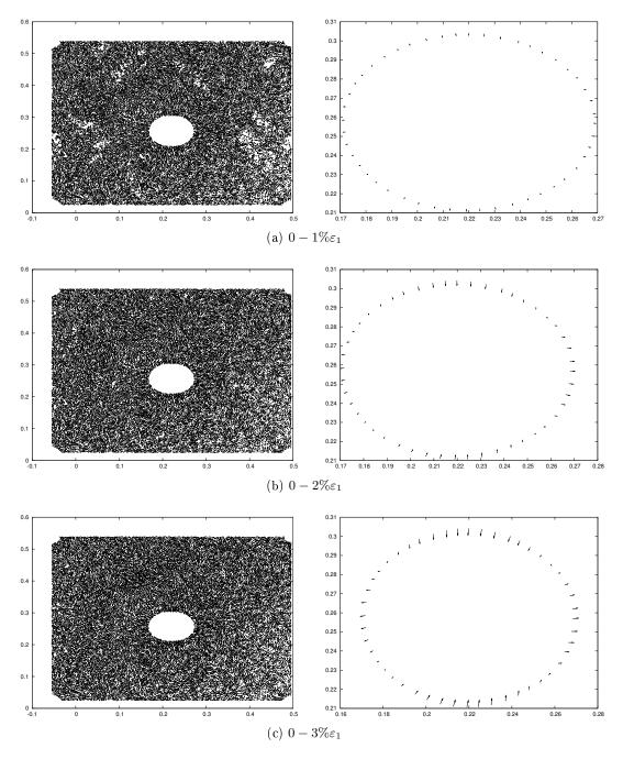
Figure D.4: PVC grains with a PVC pipe, mean field of displacement subtracted from the displacement field. The longest arrow of displacement in the figures correspond to 1cm
