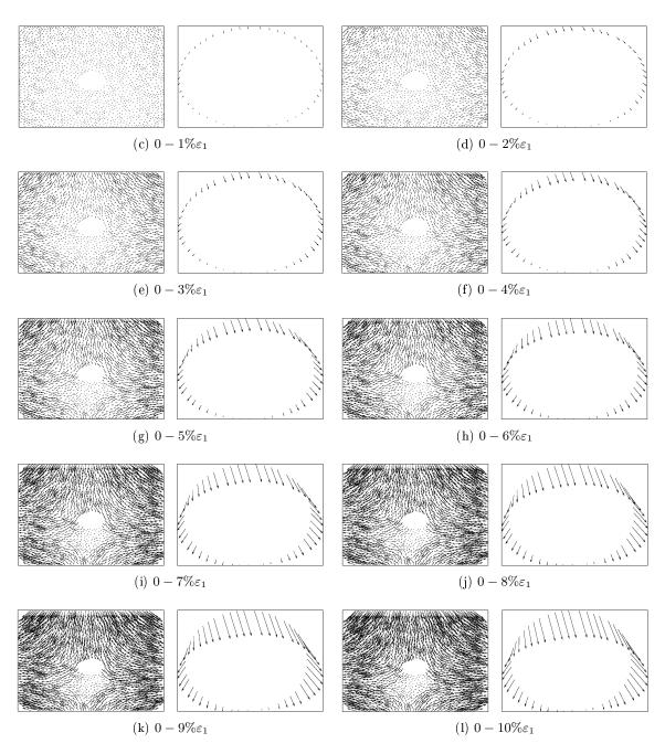
Figure 3.34: Wooden grains with a PVC pipe, displacement fields. The longest arrow of particle displacement is equal to 58mm; The biggest displacement of a point on a pipe is equal to 26mm
