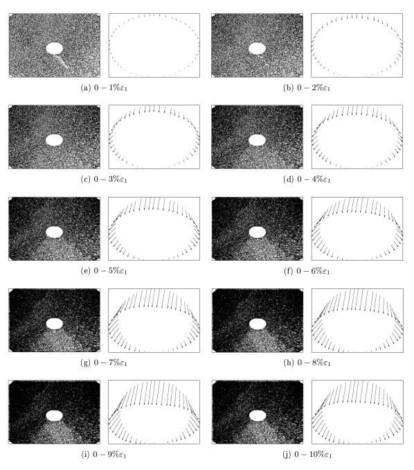
Figure 3.35: PVC grains with a PVC pipe, displacement fields. The longest arrow of particle displacement is equal to 51mm and it was reduced three times in the images for a clearer presentation; The biggest displacement of a point on a pipe is equal to 34mm
