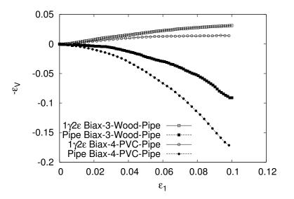
(a) Volumetric strain of the sample and pipe
