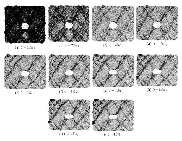
Figure 3.39: PVC grains with a PVC pipe, shear localisation. For the maximum strain the biggest symbol correspond to 2500% while the mean is equal to 32%
