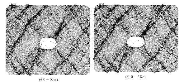
Figure D.6: PVC grains with a PVC pipe, shear localisation. For the maximum strain the biggest symbol correspond to 2500 units while the mean is equal to 32
