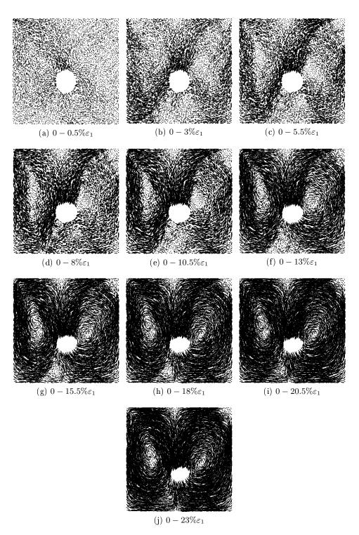
Figure 3.55: Displacement fields reduced by mean field of displacement. Clump sample with  $\alpha = 0.5$  and no friction at the boundary of the pipe
