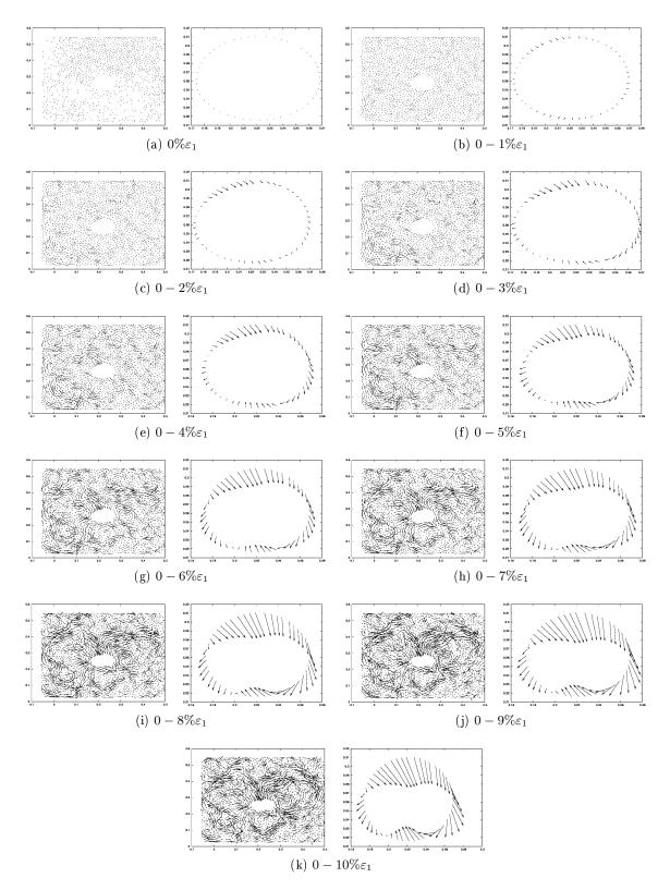
Figure 3.36: Wooden grains with a PVC pipe, a mean field of displacement was subtracted from the displacement field. The longest arrow of displacement in the figures correspond to 4cm
