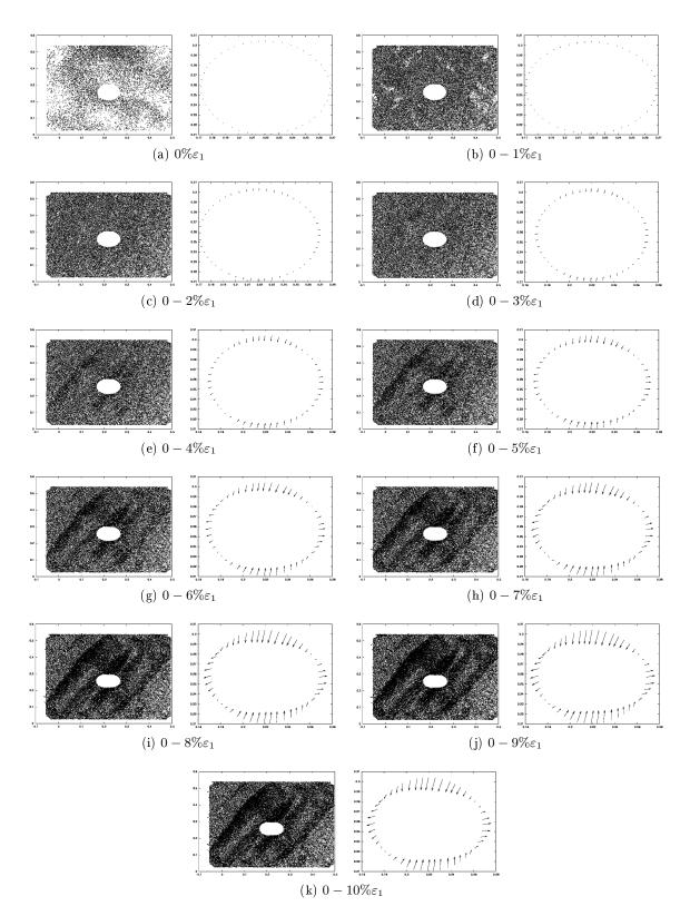
Figure 3.37: PVC grains with a PVC pipe, a mean field of displacement was subtracted from the displacement field. The longest arrow of displacement in the figures correspond to 1cm
