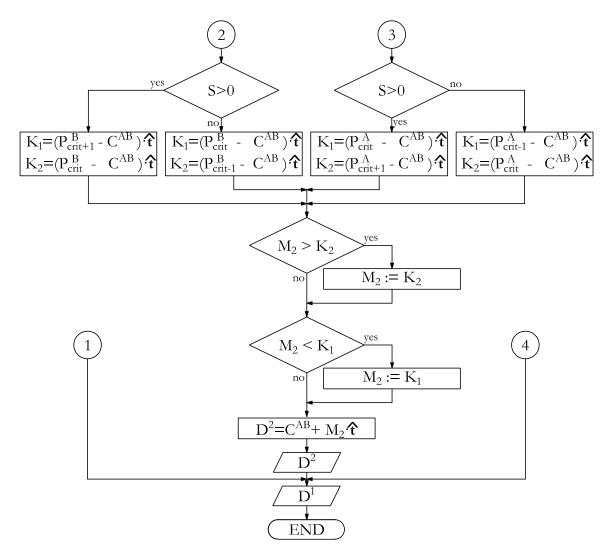
Figure A.9: Flowchart of the contact placing in Shadow Overlap method. The output is either one or two contact point geometrical positions
