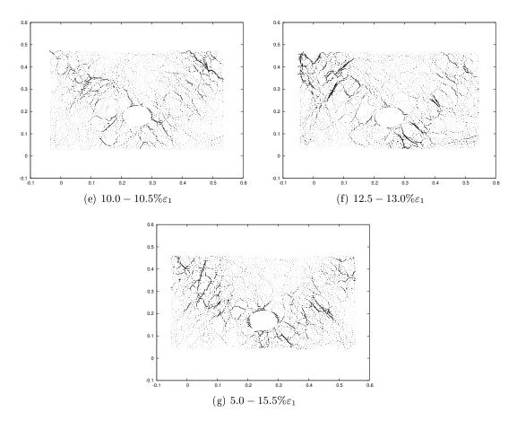
Figure E.12: Simulation of stiff pipe E = 20e9Pa with clumps  $\alpha = 0.5$  and no friction at the pipe boundary. Direction of particle stress increment
