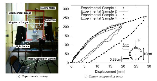
Figure 3.12: Young's modulus estimation with simple compression. The test was performed on four samples that were loaded up to different extent in the apparatus presented in Figure 3.12a. The sample was photographed in order to perform digital image correlation
