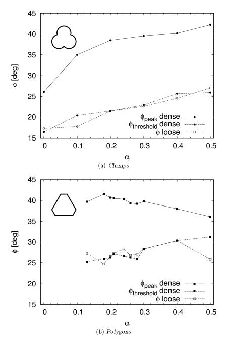
Figure 2.7: Evolution of macroscopic friction angles  $\phi$  of samples submitted to vertical biaxial compression in function of  $\alpha$ .  $\phi_{peak}$  was measured at the peak of stress while  $\phi_{threshold}$  was measured at the stress critical state
