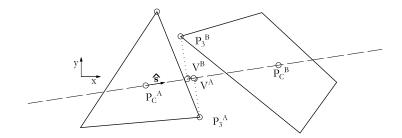
Figure A.3: Example of two neighbouring polygons that would pass the predetection test even though they are not in contact  $V^A - V^B > 0$
