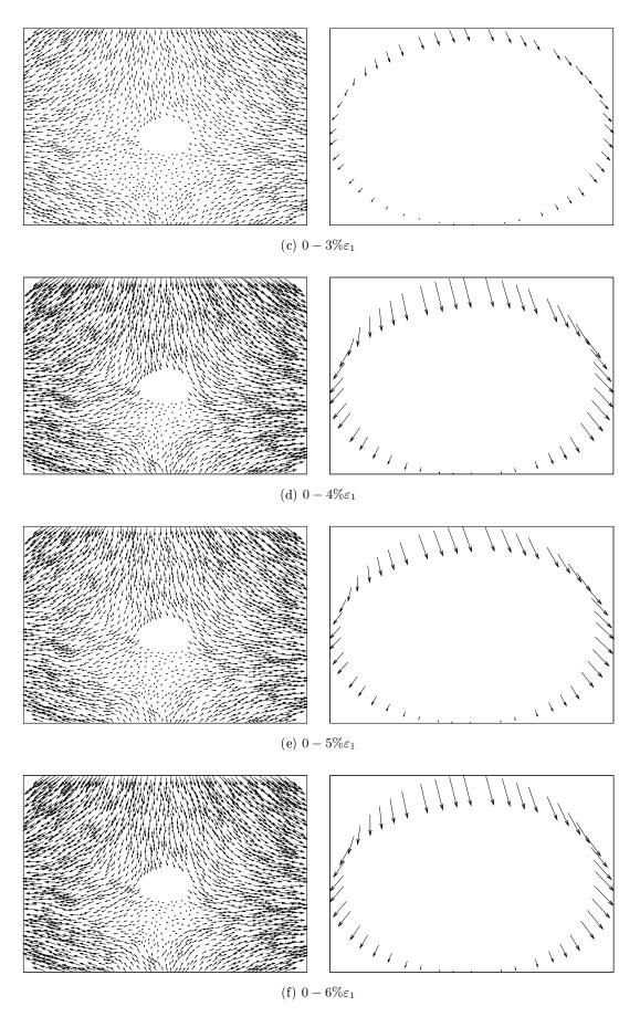
Figure D.1: Wooden grains with a PVC pipe, displacement fields
