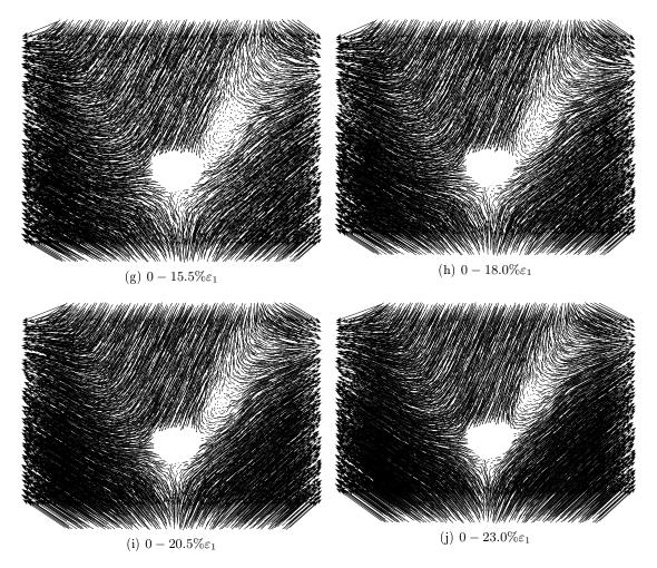
Figure E.2: Displacement fields. Clumps  $\alpha = 0.5$  without friction at the pipe boundary
