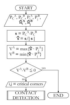
Figure A.7: Flowchart of the contact predetection. The input information needed are the positions of the corners, mass centres of the two particles and the unit vectors of the faces. As an output one learns if a contact is possible and which corners of the particles should be investigated more
