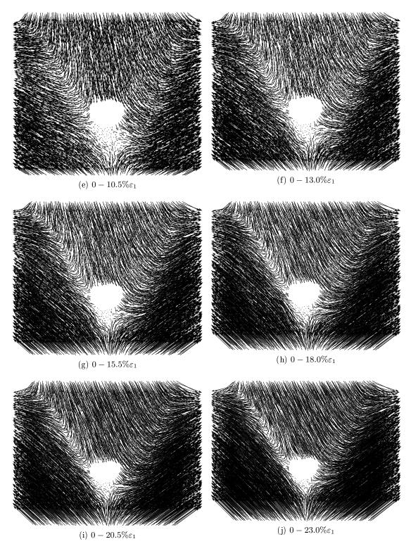
Figure E.1: Displacement fields. Clumps  $\alpha = 0.5$  with friction at the pipe boundary
