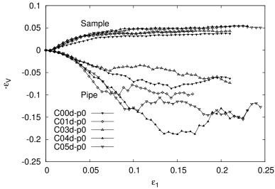
(b) Frictionless pipe-soil interface
