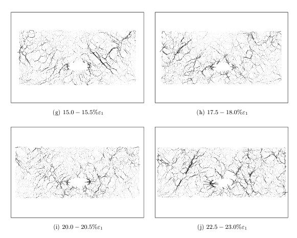
Figure E.10: Direction of particle stress increment. Clumps  $\alpha = 0.5$  without friction at the pipe boundary
