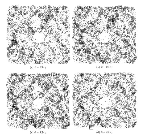
Figure D.5: Wooden grains with a PVC pipe, shear localisation. For the maximum strain the biggest symbol correspond to 300 units while the mean is equal to 35
