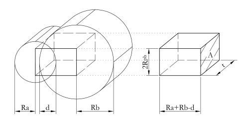
Figure 3.7: Parallel bond between two particles. The bond is a finite rectangular parallelepiped of lengths  $R_A + R_B - d$ ,  $2R^{pb}$  and t
