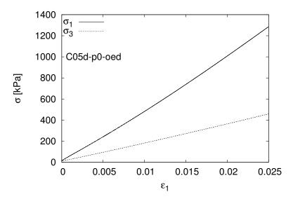
Figure 3.44: Oedometric compression stresses in a numerical simulation C05d-p0-oed
