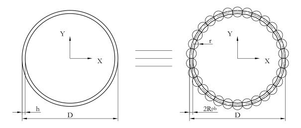
Figure 3.8: A numerical model of an elastic pipe. The model consists of a number of particles bound with parallel bonds. The distance between the bonds correspond to the thickness of the pipe while the number and diameter of the particles can be different
