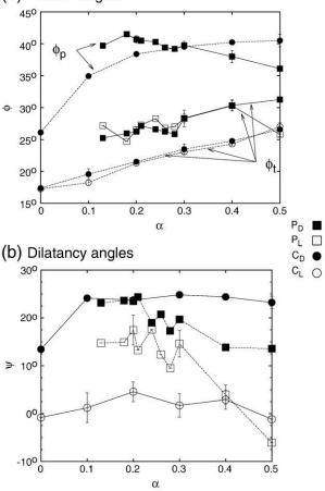
**Fig. 8.** (a) Friction angles vs.  $\alpha$  for clumps and polygons samples. The two upper curves correspond to friction angles at the peak  $\phi_p$  of dense samples. The four other curves show friction angles at the threshold  $\phi_t$ , either for dense or loose samples. (b) Dilatancy angles for all the samples; Values of the angles for dense samples were calculated at the peak, between [1.5–2.5%]  $\varepsilon_1$ ; For loose ones, the range was [6–7%]  $\varepsilon_1$ .
