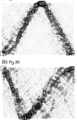
**Fig. 14.** Shear maps on dense samples made of grains with  $\alpha = 0.3$  calculated from the isotropic state to  $\varepsilon_1 = 13.5\%$ . Black square symbols are proportional to the amplitude of the second invariant of the strains  $I_{e,r}$ .
