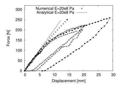
Figure 3.15: Force-displacement curve of a circular pipe simple compression. Comparison between experimental and a numerical results
