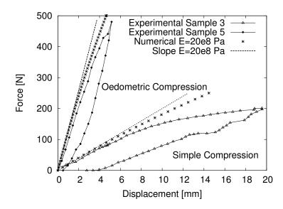
Figure 3.20: Comparison between simple and oedometric compression of pipe. The experimental results were reproduced with a numerical model. The slope of the elastic part of the curves is equal to  $3 \cdot 10^5 [Pa]$  in case of simple compression and  $2 \cdot 10^6 [Pa]$  in case of oedometric compression
