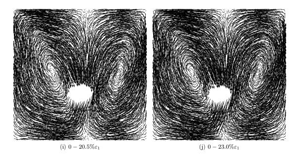
Figure E.3: Displacement fields reduced by mean field of displacement. Clumps  $\alpha = 0.5$  with friction at the pipe boundary
