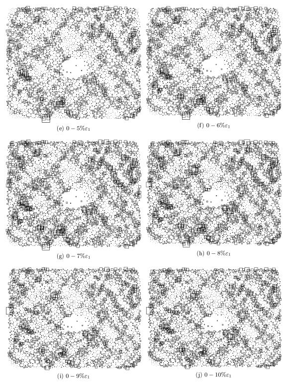
Figure D.5: Wooden grains with a PVC pipe, shear localisation
