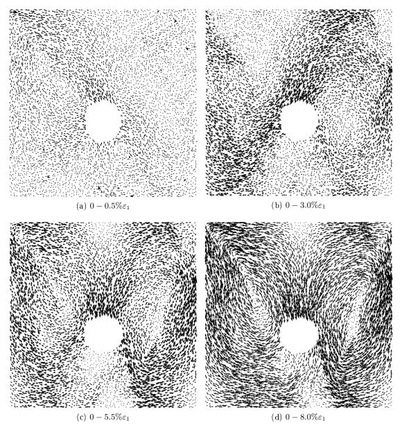
Figure E.3: Simulation of clumps  $\alpha = 0.5$  with friction at the pipe boundary. Displacement fields reduced by mean field of displacement
