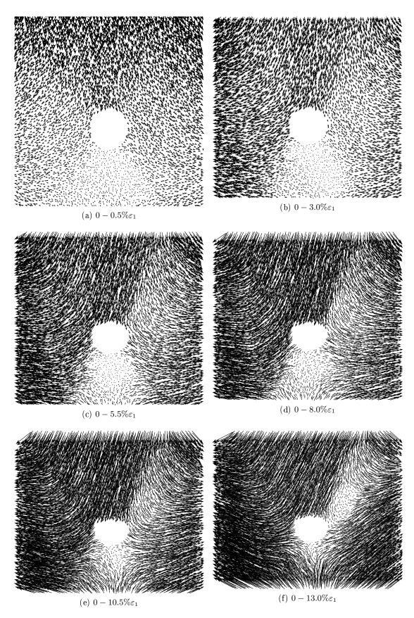
Figure E.2: Simulation of clumps  $\alpha = 0.5$  without friction at the pipe boundary. Displacement fields
