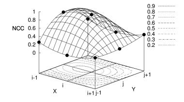
Figure 3.25: Sub-pixel refinement example. Nine discrete values of correlation coefficient are approximated with a parabolic surface in order to find a maximum value. The position of this maximum is expressed with a real number
