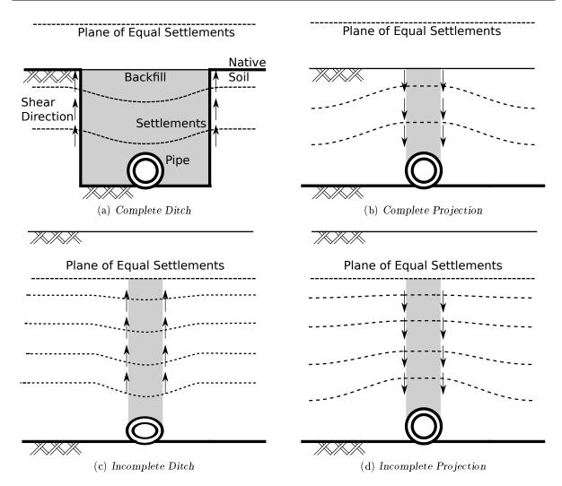
Figure 3.2: Four situations described by Marston and Spangler. Ditch and projection conditions depends whether the shearing stresses are overloading or unloading the pipe; Complete and incomplete conditions depends on the existence of a plane of equal settlements (dashed line). The native soil is denoted with a bold line, backfill level with a thin line, the soil prism in grey
