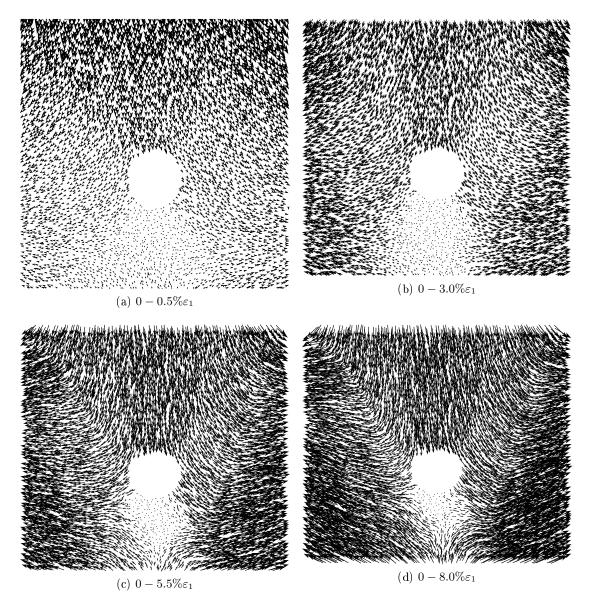
Figure E.1: Simulation of clumps  $\alpha = 0.5$  with friction at the pipe boundary. Displacement fields
