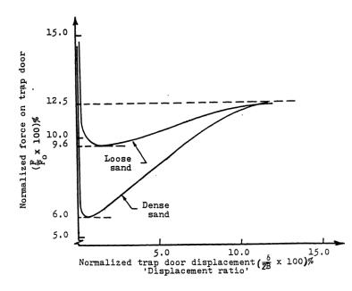
Figure 3.6: Experimental results in Terzaghi trap door experiment (after (Tien, 1996)). The force acting on the trap is quickly reducing along with the lowering of the trap and then rise again to some residual level
