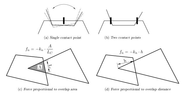
Figure 1.10: Difference between a standard polygon contact treatment (left) and the one introduced in Moreau's Shadow Overlap Method (right). More on contact force computation in Section 1.7
