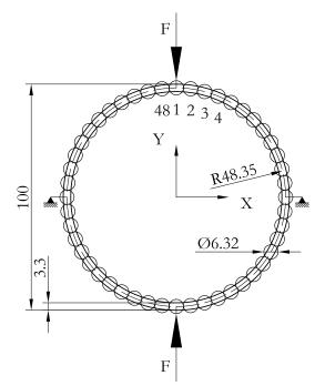
(a) Pipe geometry used in the validation of the numerical model. The model is divided into 48 sections
