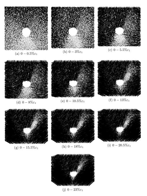
Figure 3.53: Displacement fields of a clump sample with  $\alpha = 0.5$  and no friction at the boundary of the pipe
