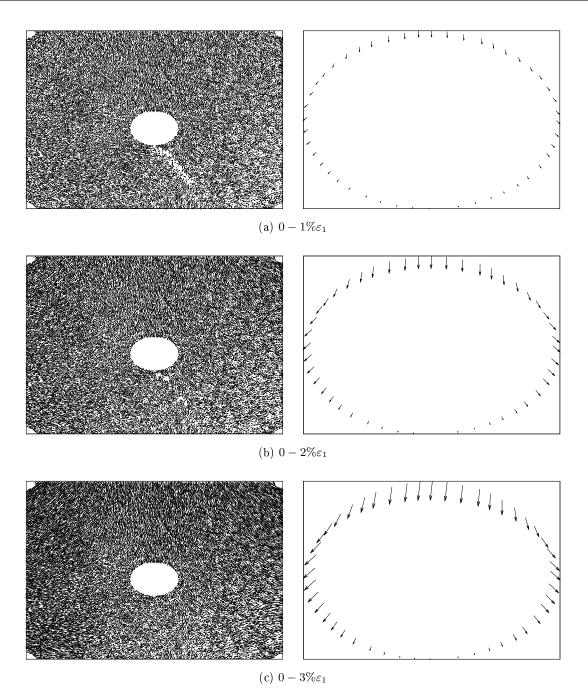
Figure D.2: PVC grains with a PVC pipe, displacement fields. The longest arrow of particle displacement is equal to 21mm and it was reduced three times in the images for a clearer presentation; The biggest displacement of a point on a pipe is equal to 34mm
