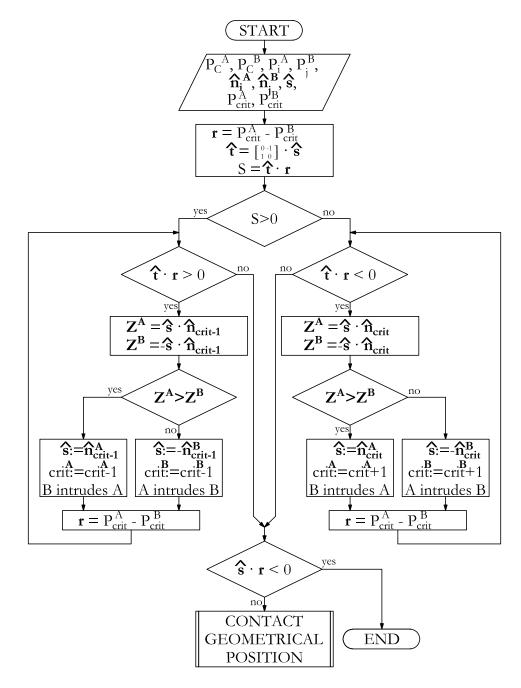
Figure A.8: Flowchart of the contact detection phase. Apart from the basic information about the particles carried from the predetection phase, the input consists of the vector  $\hat{s}$  direction and the initial critical corner numbers
