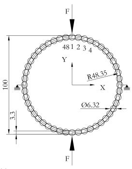
(a) Pipe geometry used in the validation of the numerical model. The model is divided into 48 sections
