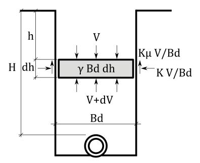
Figure 3.1: The basis of Marston approach, a pipe in a ditch and the loads acting on a strip of soil above it
