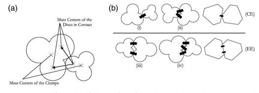
Fig. 2. Contacts between the particles; contact definition and classification. (a) Definition of a contact between clumps. Normal contact vector connects the centers of the discs in contact. (b) Various types of possible contacts between clumps. Analogy between clump and polygon contacts: corner-to-edge (CE) and edge-to-edge (EE) groups. Note that for a contact between two polygon edges two contact points are considered while only one if there is a contact between a corner and an edge.
