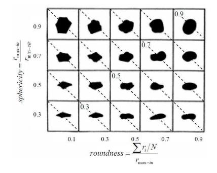
Figure 1.2: Chart presenting some natural grain shapes with different values of sphericity and roundness, originally from (Krumbein and Sloss, 1951), modified by (Cho et al., 2006)
