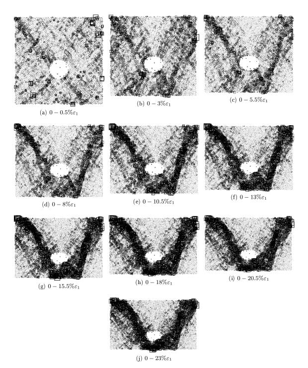
Figure 3.56: Shear localisation maps of a clump sample  $\alpha = 0.5$  with friction at the pipe boundary
