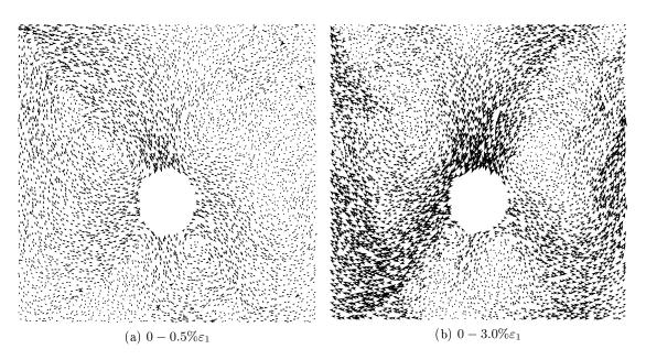
Figure E.4: Simulation of clumps  $\alpha = 0.5$  without friction at the pipe boundary. Displacement fields reduced by mean field of displacement
