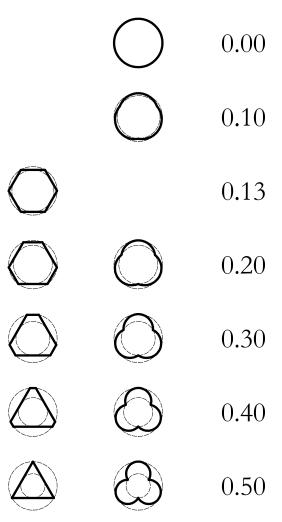
Figure 2.6: Particle shapes used in the study. The outer radius of particles  $R_1$  is constant. The left column presents polygonal grains, the right one clumps. Values of shape parameter  $\alpha$  are given for each shape. Note the absence of polygons  $\alpha = 0.00$  and  $\alpha = 0.10$ , as well as clumps  $\alpha = 0.13$
