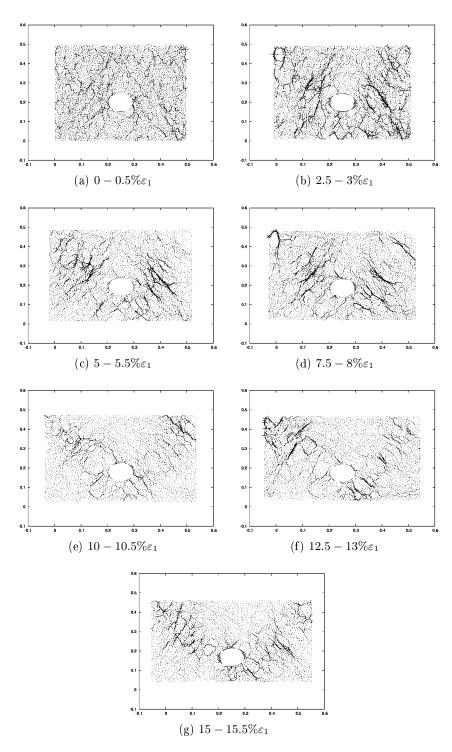
Figure 3.65: Direction of particle stress increment during biaxial compression of a clump sample with  $\alpha = 0.5$  and frictionless pipe with Young's modulus E = 20e9Pa
