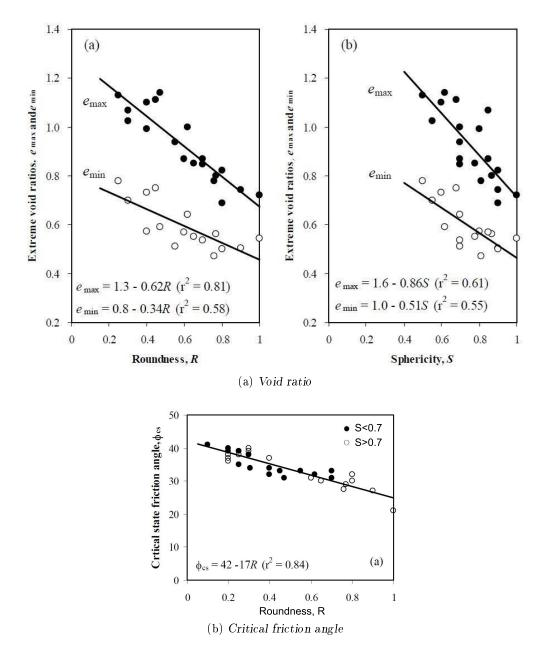
Figure 1.4: Relationship between particle roundness and sphericity, and the void ratio and friction angle for various sands, after (Cho et al., 2006)
