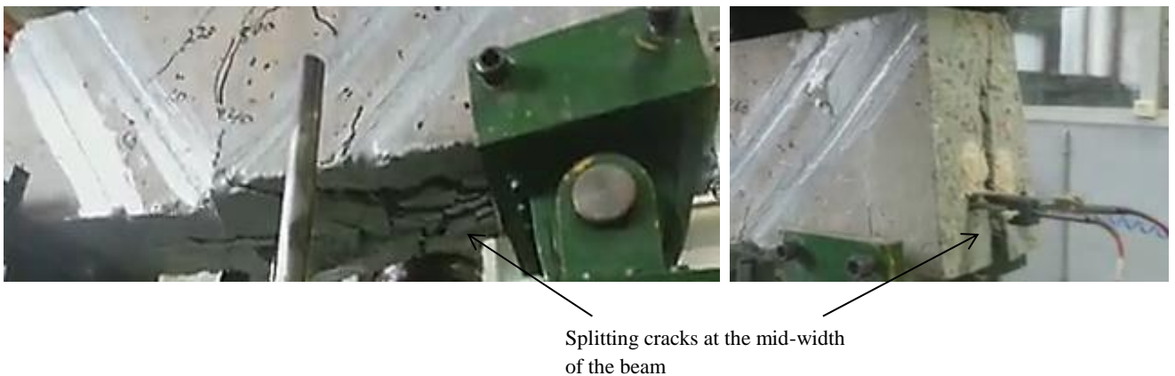
Figure 4 - 7 Tensile steel bars slip occurred in non-shear repaired beams A1T-SB and A1CL3-SB
