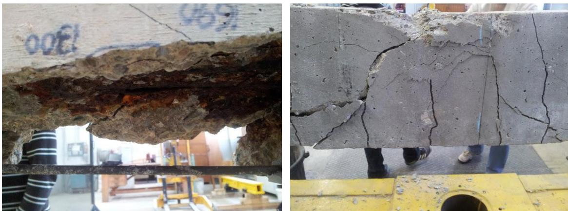
a) A1CL3-R Corroded Beam
