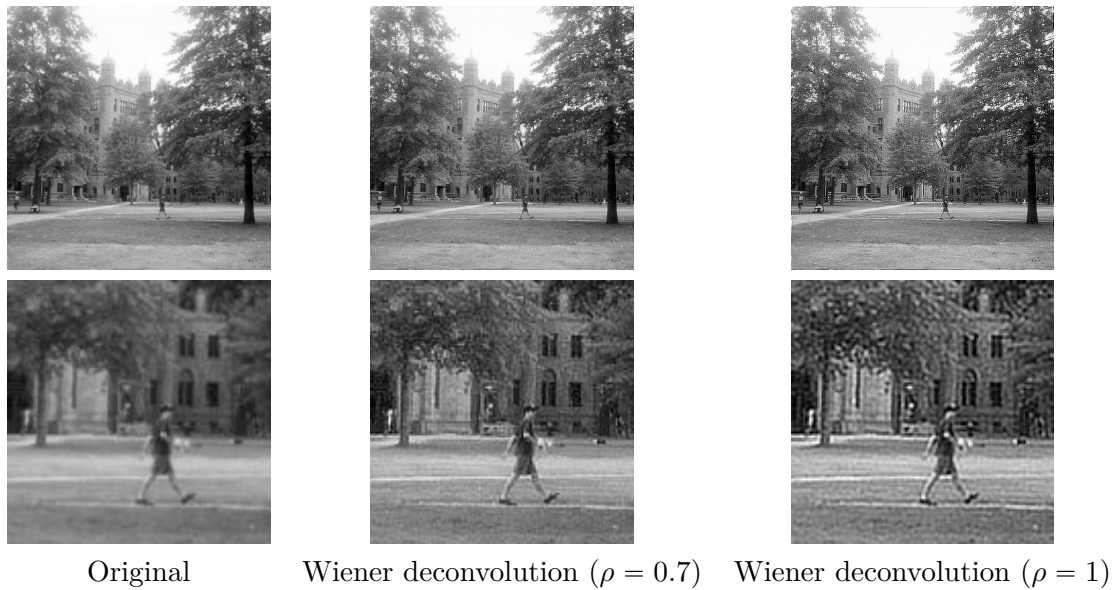
Figure 4.9: Parametric blind deconvolution using sharpness indices. On the first row, we can see the original Yale image (left), and two Wiener- H^1 deconvolution results obtained with a kernel width of \rho = 0.7 (middle) and \rho = 1 (right). Close-up views of these three images are shown on the second row. The value \rho = 0.7 , which maximizes the sharpness indices SI and S (see Fig. 4.8), corresponds surprisingly well to the desired critical value that rules the transition between blur and ringing.
