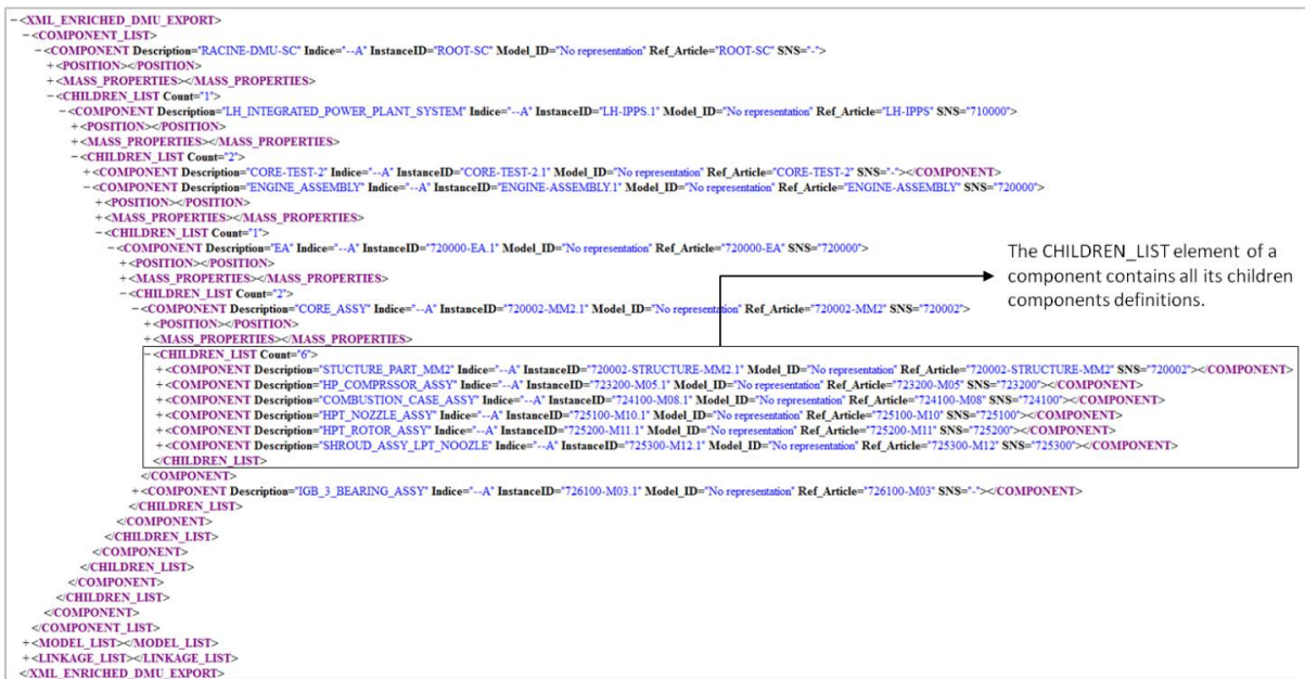
Figure 186: the CHILDREN_LIST elements recursively capturing the children components for each DMU constituent
