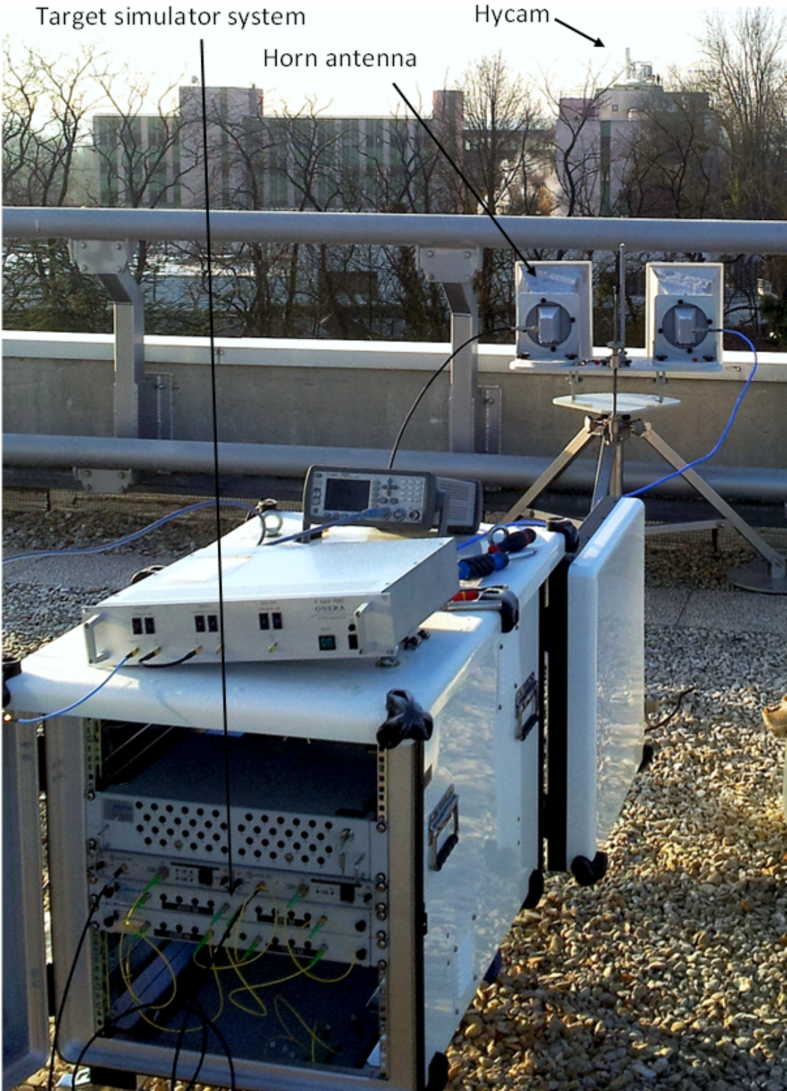
Figure 5.1: Installation for the target simulator, localized at 250 m of Hycam
