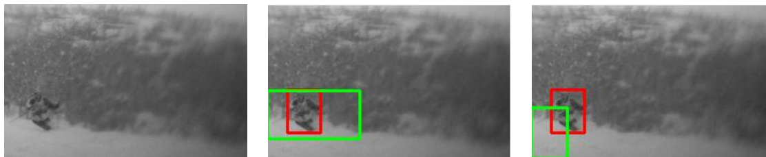
FIGURE 4.6 – Example of salient region segmentation with the Skiing sequence. From left to right : input frame ; detection with Binary Threshold and with Motion Priority fusion techniques. Red box indicates ground truth and green box indicates the detected salient region.
