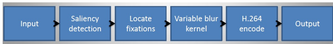
FIGURE 2.9 – Video compression procedure using saliency detection method
