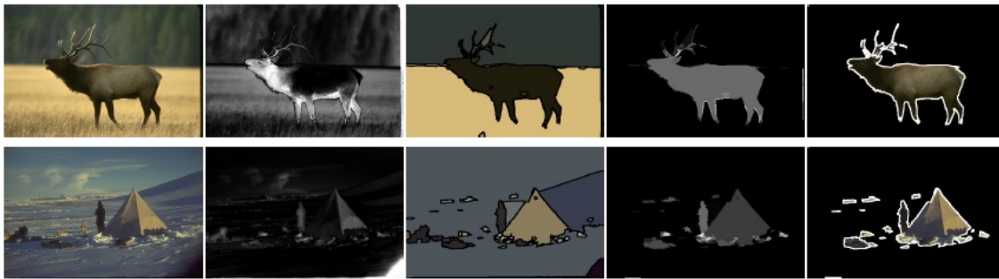
FIGURE 2.7 – Example of image segmentation using visual saliency. From left to right : original image, obtained saliency map, mean-shift segmentation, and segmentation based on saliency values (last two columns). Source [3].
