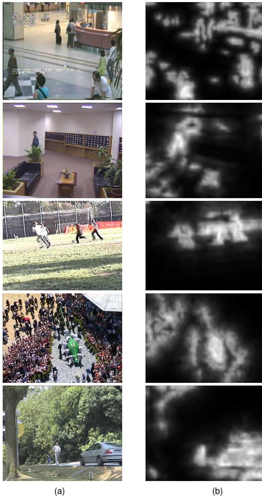
FIGURE 3.15 – Examples of spatio-temporal saliency detection map using color and texture features. (a) Original frame (b) Spatio-temporal saliency map.
