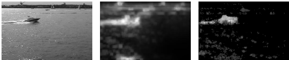
FIGURE 4.9 – Examples of static and dynamic saliency detection on good color contrast and motion contrast boats sequence. From left to right : Original frame , Static saliency and Dynamic saliency .
