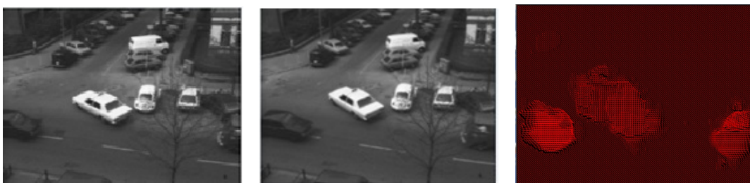
FIGURE 3.4 – The dense optical flow estimation on successive video frames. From left to right : original video frames and motion estimation of each pixel.
