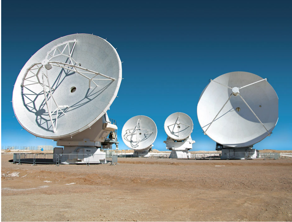
Figure 2.6.: Parabolic reflector antennas used as part of Atacama Large Millimeter Array (ALMA) antennas (© ALMA (ESO/NAOJ/NRAO), W. Garnier (ALMA))
