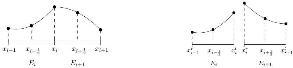
FIGURE 1.4 – Example of parabolic finite element approximation in one dimension : continuous (left) and discontinuous (right) cases.
