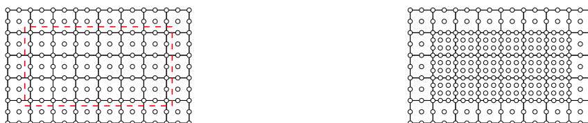
(a) A grid composed exclusively of quadrangular Q2 with the selected region to refine in red. (b) The order of the elements in the selected region has increased.
