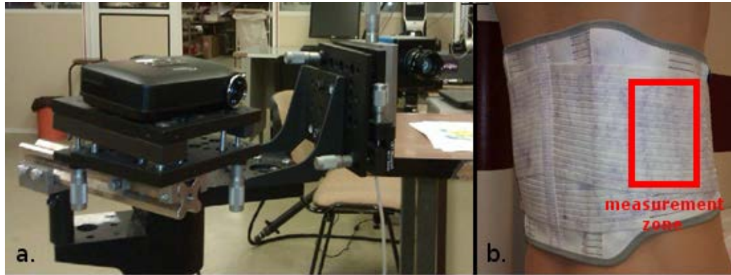
Figure 2.6 – Representation of a. optical system and b. mannequin wearing lumbar belt
